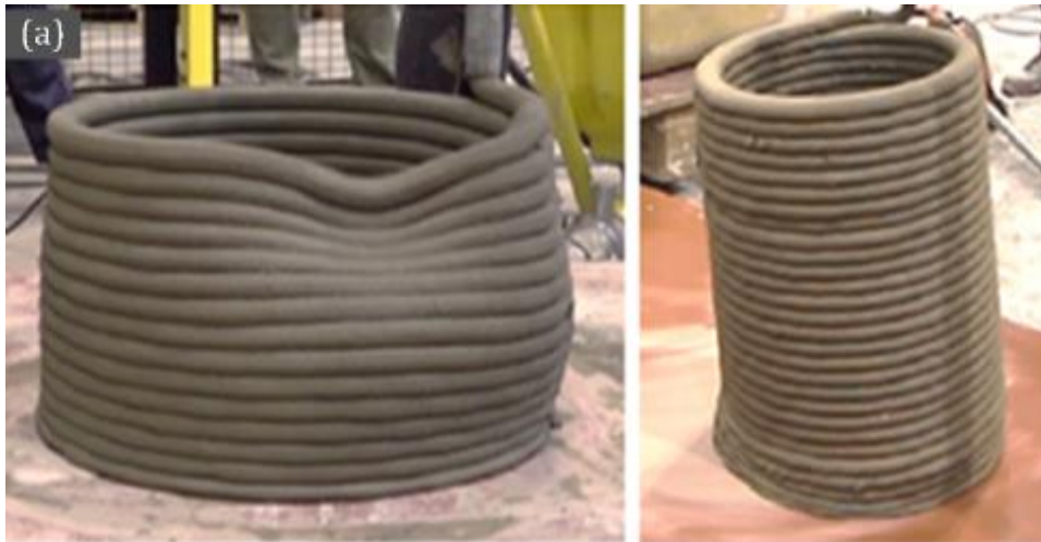
Joonis 1.10 Vasakul elastne paindumine, paremal plastiline purunemine [24]
