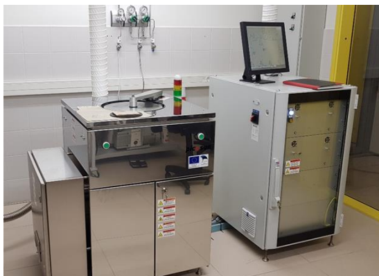
Picture 1 Picosun R200 reaction chamber on left and main computer on right. [43]
