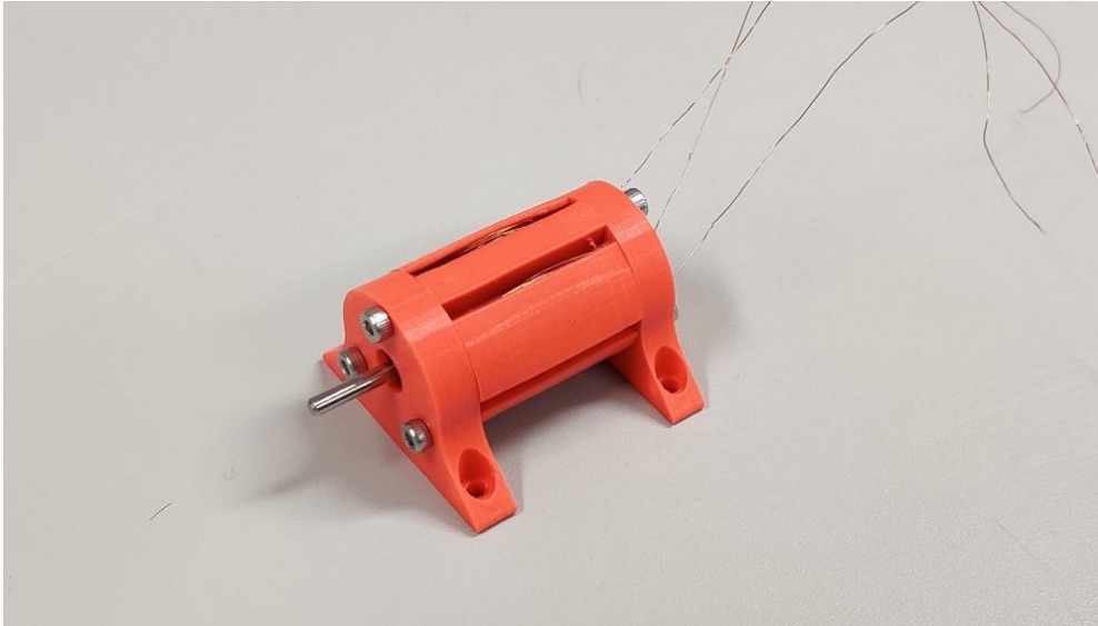
Figure 2.2 Prototype coreless machine used in thesis
