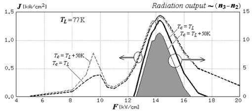
**Figure 3** Current density and expected laser radiation output (in arbitrary units) versus applied field.
