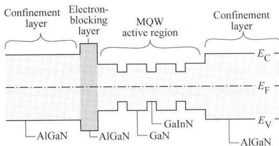
Figure 1.6: An example application of quantum wells in Light Emitting Diodes. The multiple quantum wells act there as an active region and increase the efficiency of light generation. Source: Fig. 4.14 (a) in [18]
