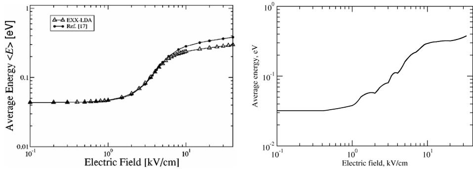
Figure 3.6: Comparison of the original and the interpolated dependence between average energy and electric field at 300 K in GaAs (source: Fig. 4 in [24]).
