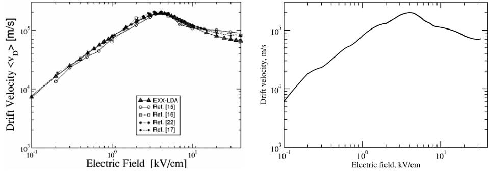
Figure 3.5: Comparison of the original (left) and interpolated (right) dependence between drift velocity and electric field at 300 K in GaAs (source: Fig. 3 in [24]).
