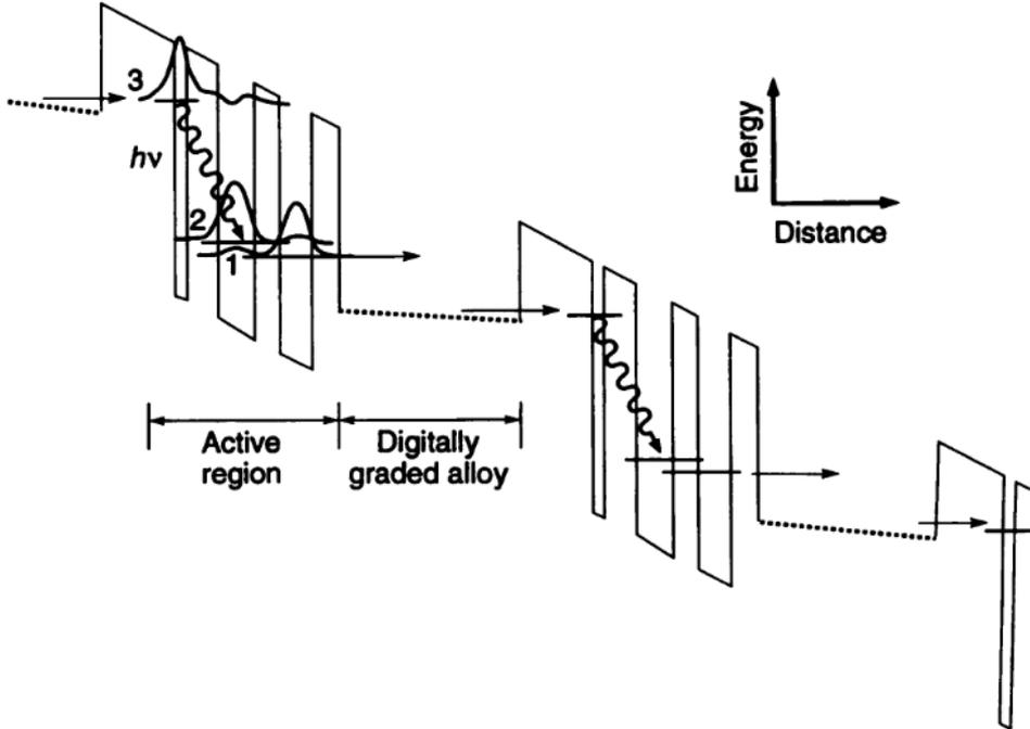
Figure 1.7: A conduction band diagram of the Quantum Cascade Laser. Only two periods of the multiple layer structure are shown here. Numbers show the energy levels of electrons counting from the bottom of one period. [9]
