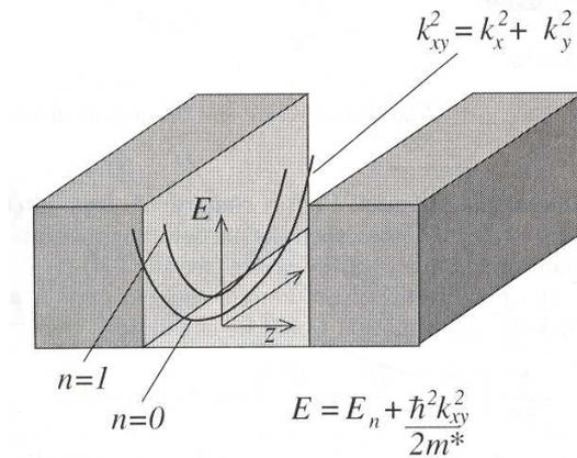
Figure 3.1: In-plane dispersion curves and the subband structure. Source: Fig. 2.5, page 22 in [3].
