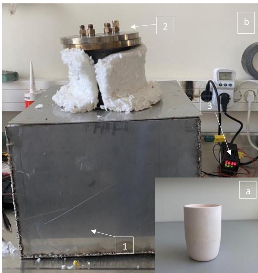
**Figure 2.1.** Alumina crucible (a) and the stainless steel reactor (b) (1-main body of the reactor, 2- gas inlet/ outlet and 3- temperature controller)
