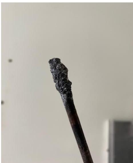
**Figure 3.5.** Carbon produced from electrolysis in Li-K carbonate electrolyte on stainless-steel 304 electrode
