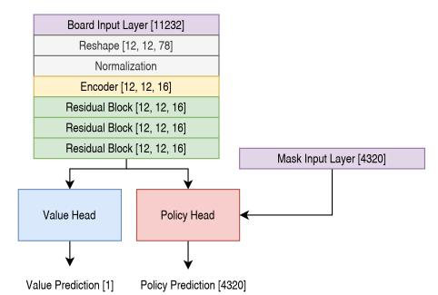
Figure 10. The architecture of PlayerZero model. Numbers in square brackets represent the shape of data in the layers.
