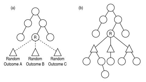
Figure 9. Determinization with Random nodes in MCTS. (a) An action with a random outcome is marked with "R", the triangles represent random nodes corresponding to each of the possible outcomes. (b) After expansion of the random nodes, the tree structure continues as before.
