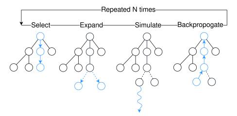
Figure 1. An image illustrating the 4 phases of MCTS: Selection, Expansion, Simulation, and Backpropagation.
