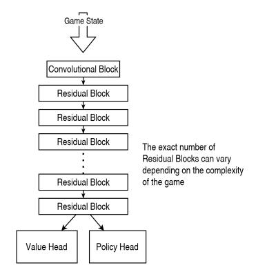
Figure 2. A simplified diagram of the AlphaZero DCNN model architecture.
