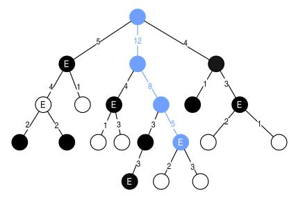
Figure 8. A diagram demonstrating how the optimal series of actions is recovered from MCTS with varying length turns. The numbers on the connections represent the number of times the nodes have been visited. The blue highlight shows the optimal sequence of actions.
