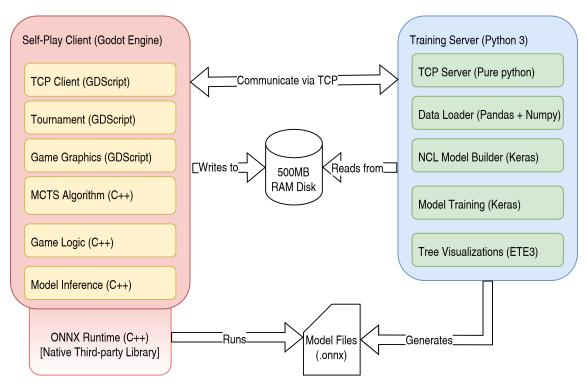
The architecure of the two components and how they integrate is shown in Figure 6.
