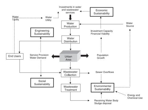
*Figure 6. Urban water sector system. Solid lines represent water flows, and broken lines represent relevance to sustainability (adapted from Sahely et. al 2005).*
