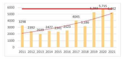
Figure 18 Carbon dioxide (CO<sub>2</sub>) emissions at Tallinna Vesi WWTP (at the limit of 5789.49 t/yr)
