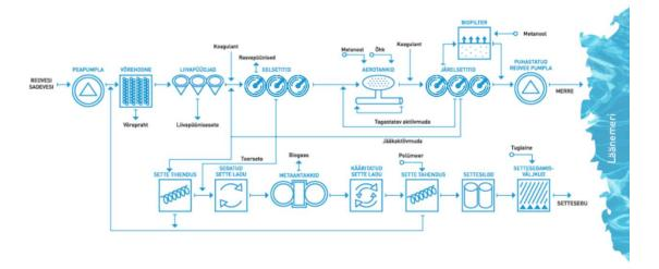
Figure 10. Wastewater treatment process at Paljassaare wastewater treatment plant (Tallinna Vesi AS, 2021)
