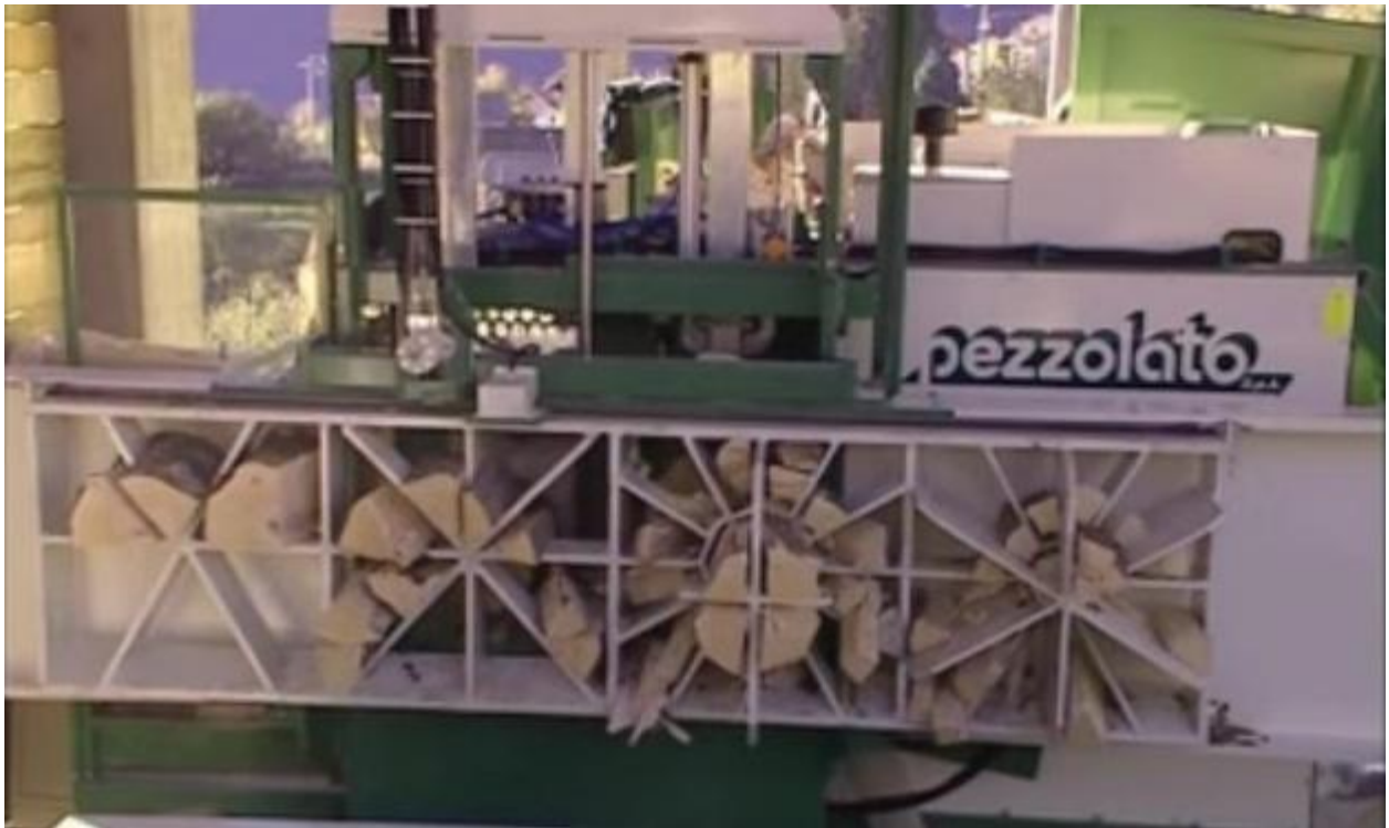
Pezzolato TLC 1400 firewood processor with horizontal multiple splitting grid. The splitting grid is movable in both directions: up and down, left and right. Source: Youtube video [39].
