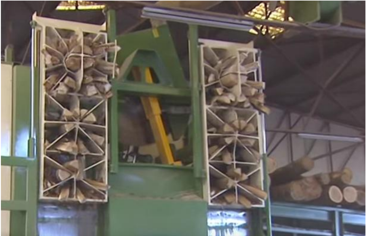
Pezzolato TLA 150 firewood processor with multiple splitting grids [38].
