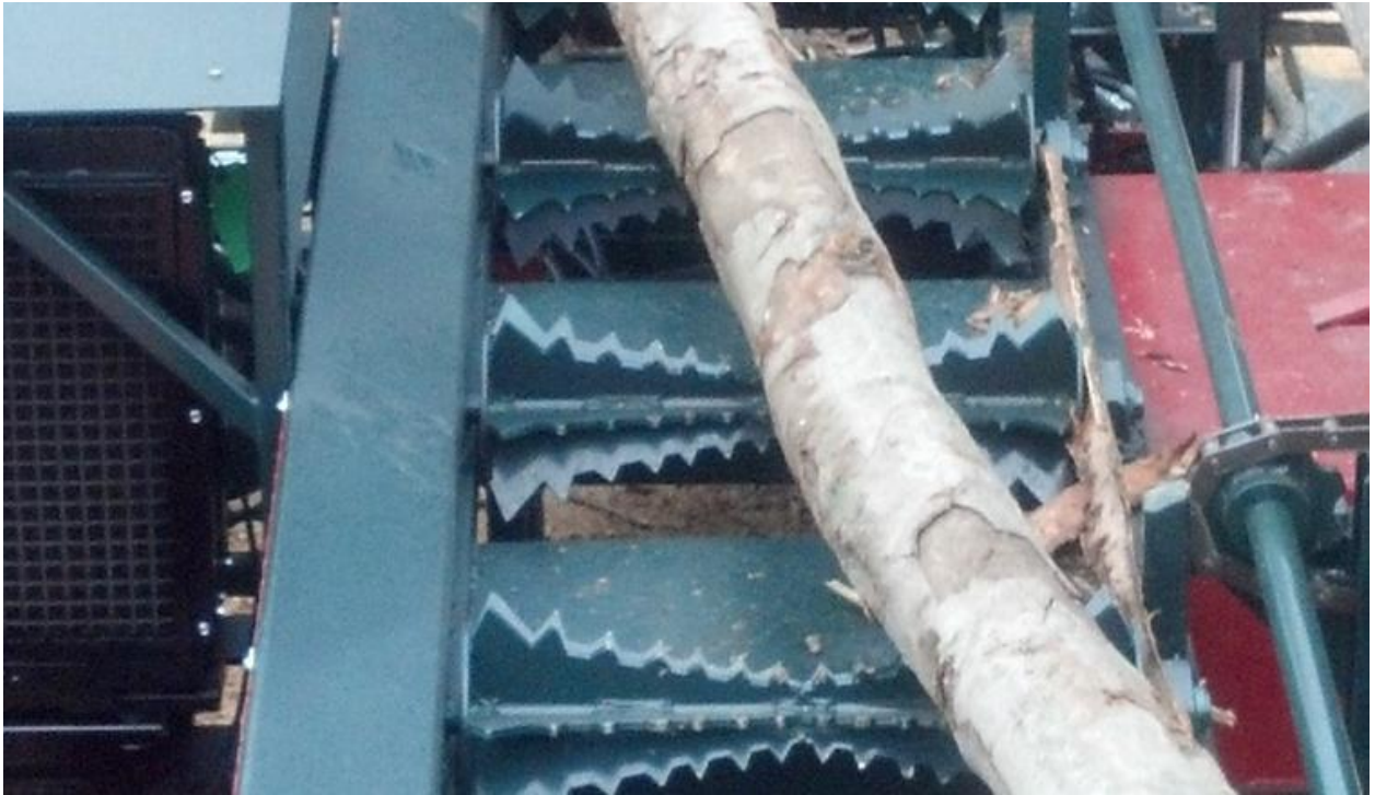
Log feeder with rotating rollers [16]
