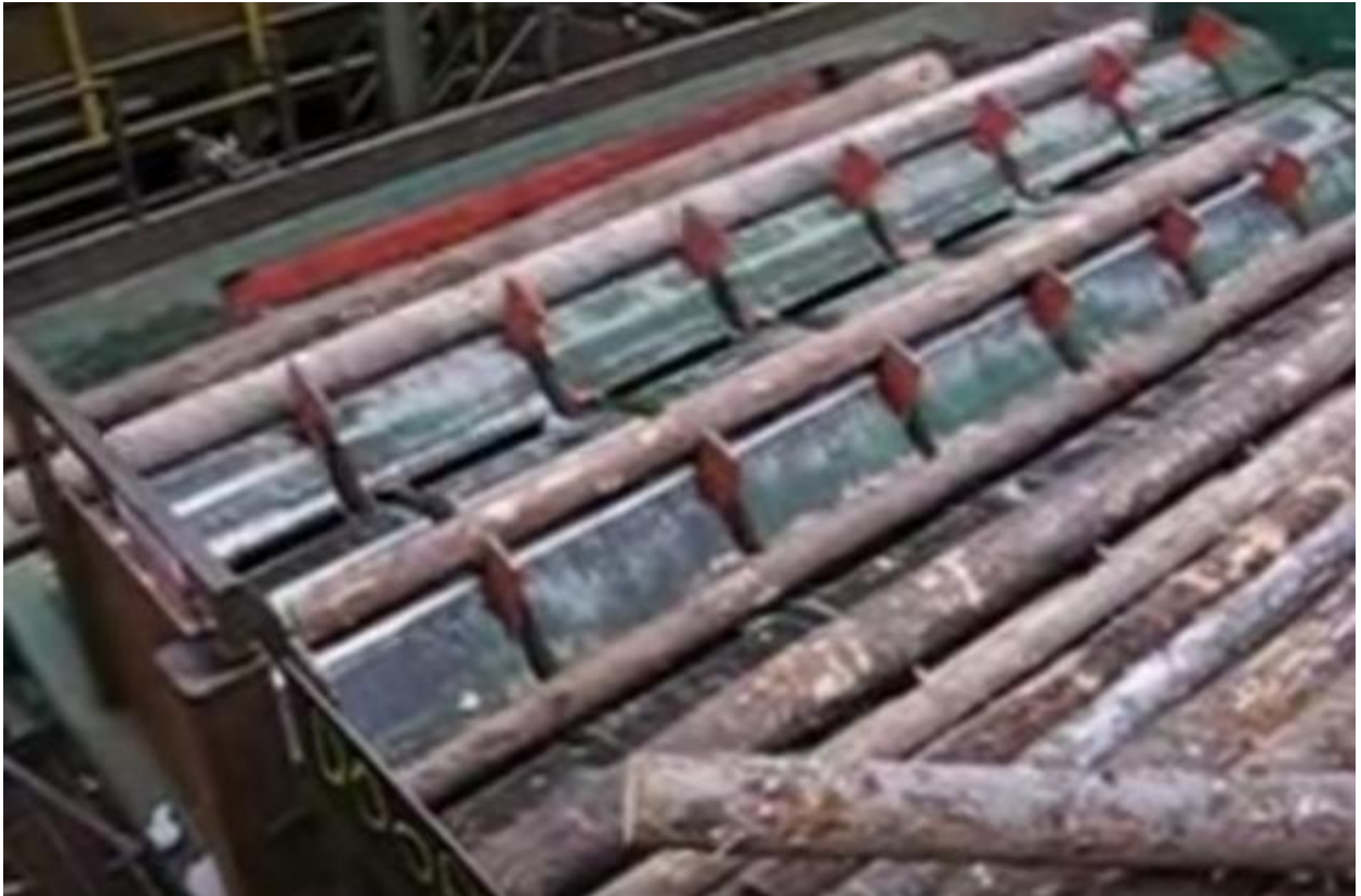
Rotary log singulator. Source: screenshot from video [5], https://www.youtube.com/watch?v=IDmUir8edRY .
