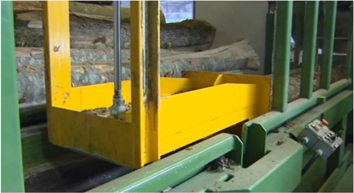
Pezzolato TLA 150 push plate feeder unit [19]
