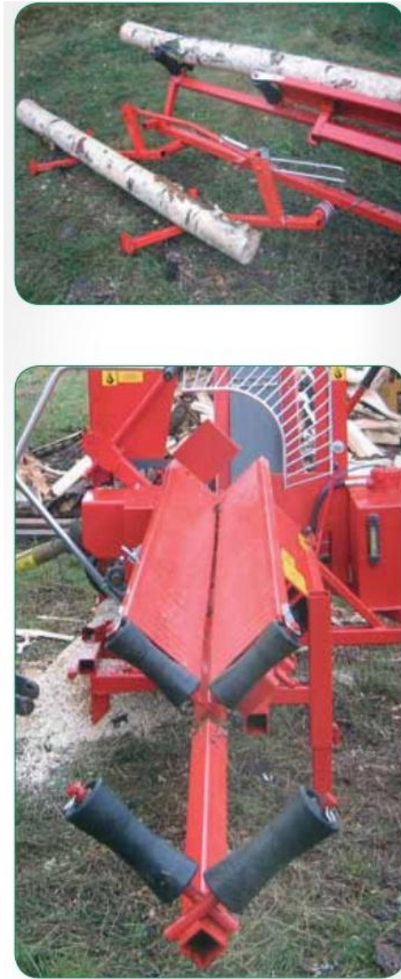
Mastersplit WP 30 and 36 firewood processor with sliding deck log feeder [17].
