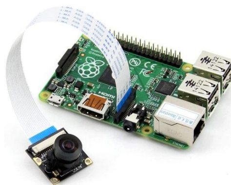
Figure 3: RPi Fisheye Lens Camera attached to a RPi CSI-interface [38]
