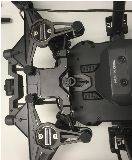
Figure 9: Attachment of Mounting Mechanism to Drone. (Before and After)
