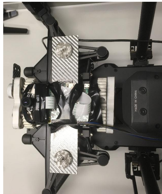
Figure 9: Attachment of Mounting Mechanism to Drone. (Before and After)
