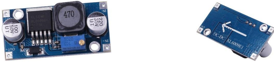
Figure 6: Voltage-regulator Module (top-view and bottom-view) [39]
