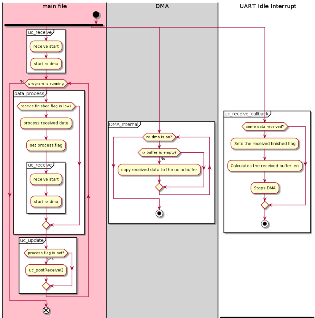
Figure 5.15 UART Communication receiving flowchart
