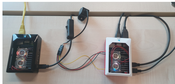
Figure 10. Raspberries for data management and gateway.
