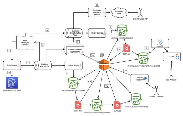
Figure 1. Architecture of existing system
