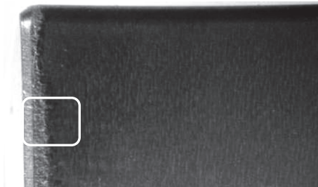
Fig. 2. SEM photograph of punch cutting edge (after 80 000 cycles). Figure 3 will show a close-up of the worn surface indicated in the white box
