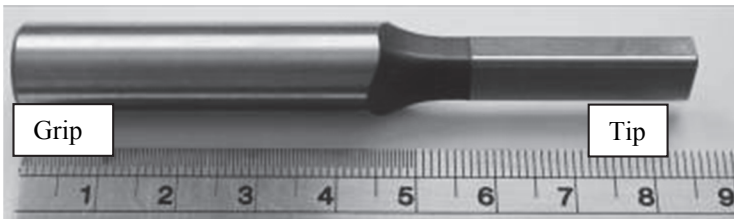
Figure 2.1 Un-coated GR-punch used in the field tests in Paper I and Paper A (Paper A).
