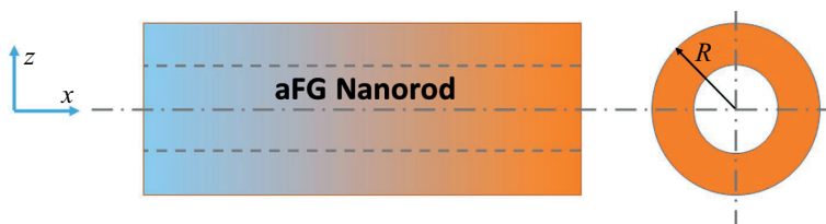
Fig 1. Axially graded nanorod continuum model.
