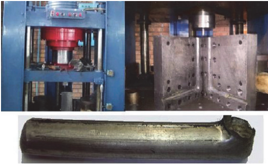
FIGURE 3.—Hydraulic press set-up, ECAP die, and sample (color figure available online).
