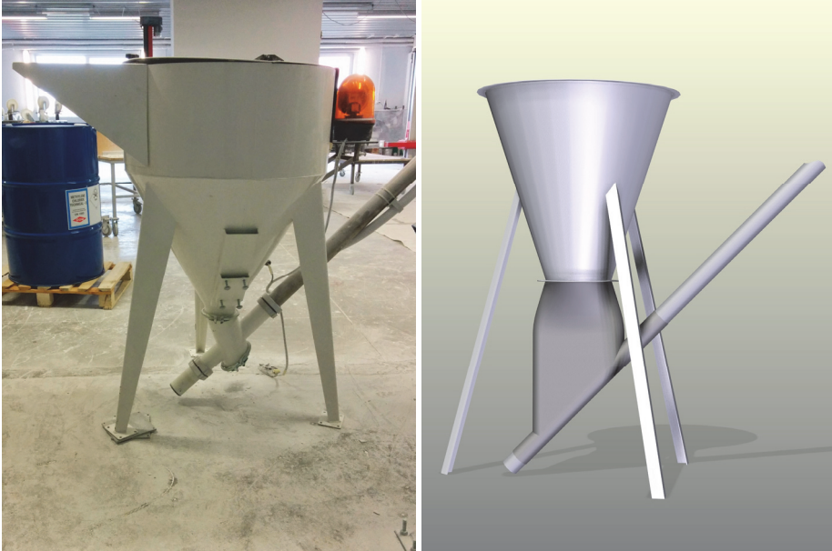
Figure 4.9 Hopper redesign: left old design and right improved design
