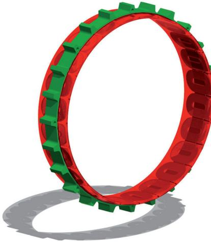
Figure 3.5. Schematic of the stator.
