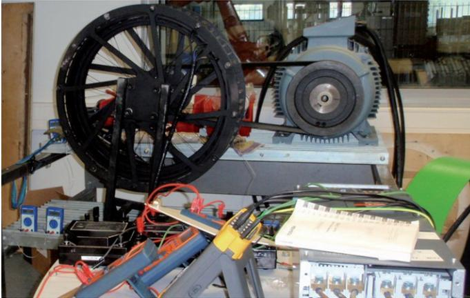
*Figure 3.6. Test bench of the generator*
