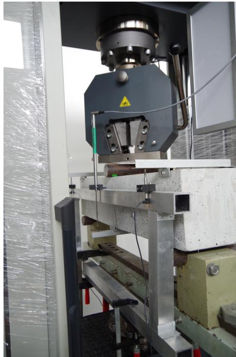
Figure 18: Photo of the bending test showing a beam sample in the testing machine with the frame for displacement measurements and displacement sensors. The figure is reproduced from Publication I.
