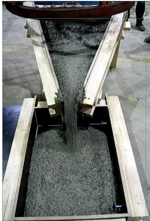
Figure 12: Casting of a small plate using a bucket and half-funnel. The figure is reproduced from Publication II.
