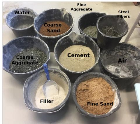
Figure 10: The ingredients of the SFRSCC mixture.
