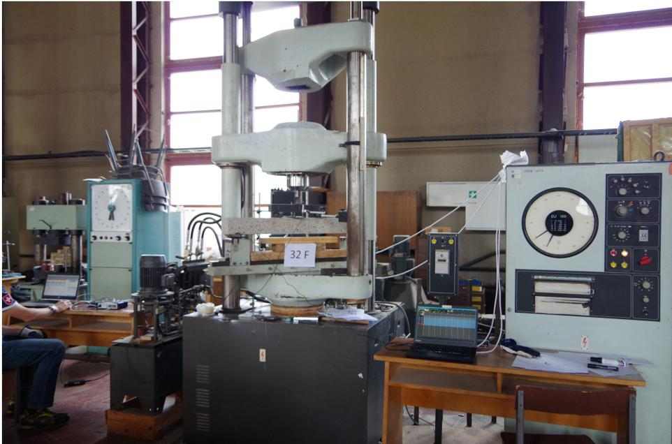
Figure 19: Four-point bending test setup with a beam sample. The figure is reproduced from Publication III.
