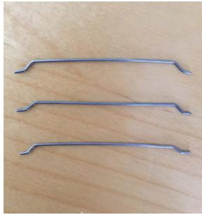
Figure 11: Hooked end steel fibers.
