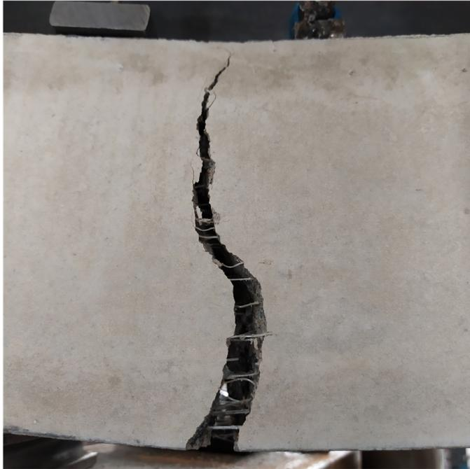
*Figure 2: Fiber concrete with visible fibers in the crack.*
