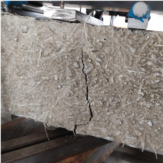
*Figure 3: The restraining effect of the fibers in the crack.*
