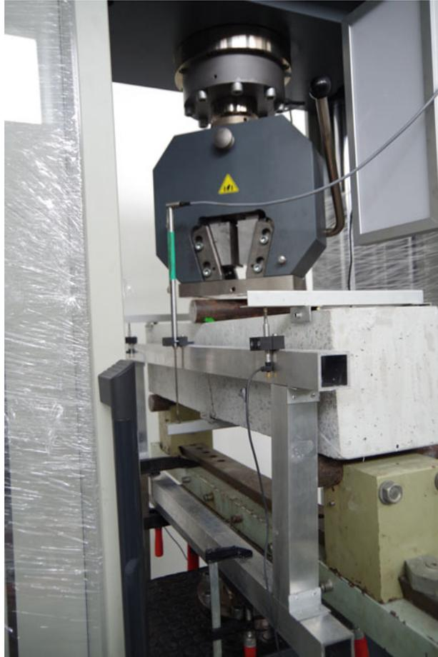
The recorded force-displacement curves are presented in Fig. 8 where the maximum force value before cracking is  $F_1 = 45.36$  kN,  $F_2 = 44.06$  kN and  $F_3 = 43.18$  kN for beams 1, 2, and 3, respectively. The formula to calculate the maximum bending stresses in a cross-section is  $\sigma^{M_y} = \frac{M_y}{W_y}$  that we apply in the cross-section  $C$  where the bending moment is given by  $M_y = FL/4$  and the section modulus is given by  $W_y = (wh^2)/6$ .
