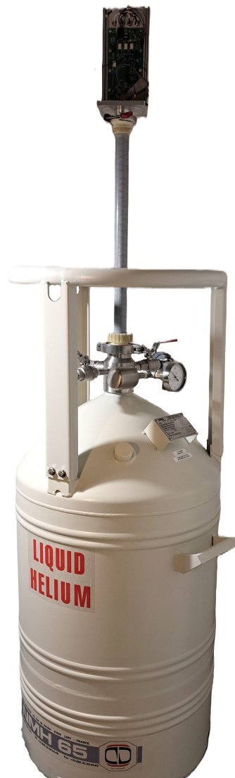
Figure 7.1: VTTs setup used for 4.2K measurements, where dipstick is inserted into the Dewar filled with liquid helium. The top part of the dipstick is a cage where room temperature electronics are situated. Signal lines are fed from the bottom of the dipstick all the way to the room temperature electronics, inside the fiberglass tube.
