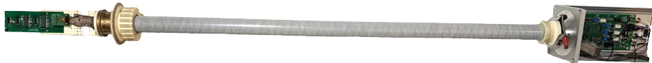
Figure 2.4: Dipstick for SQUID measurements in VTT. On the left is a plastic cold head for attaching the sample and connecting it to the signal lines, going through the narrow tube all the way to the right, through the feed through, to the room temperature electronics.
