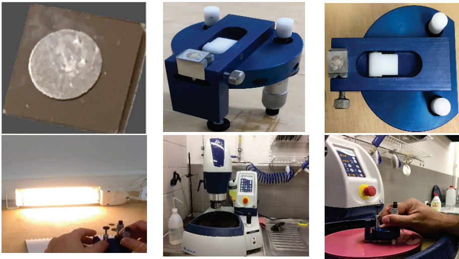
Fig. 4.33: Photograph of the bonded high-temperature Al-foil/4H-SiC SBD. The sample thinning prepared by gluing the assembly and polishing and grinding with a diamond disk (from left to right).
