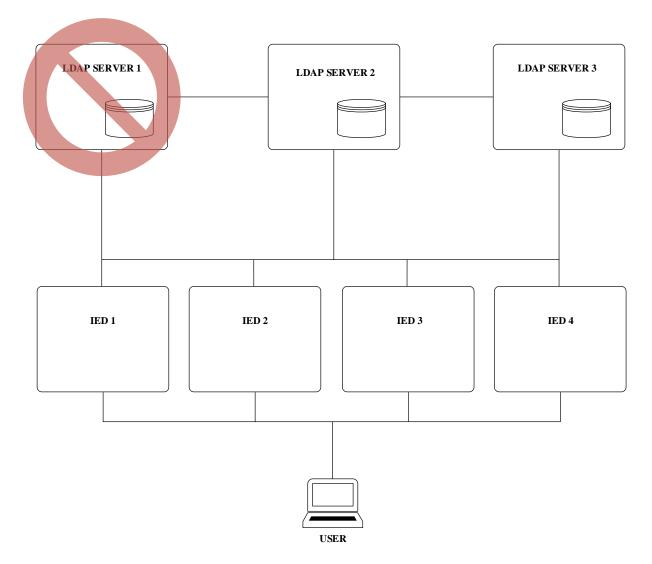
Figure 3.5.2 Logical drawing of multiple LDAP server setup
