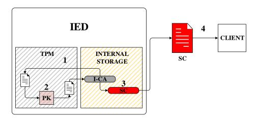
Figure 4.3.1 IED with secure storage and the I-CA (PK on the TPM)
