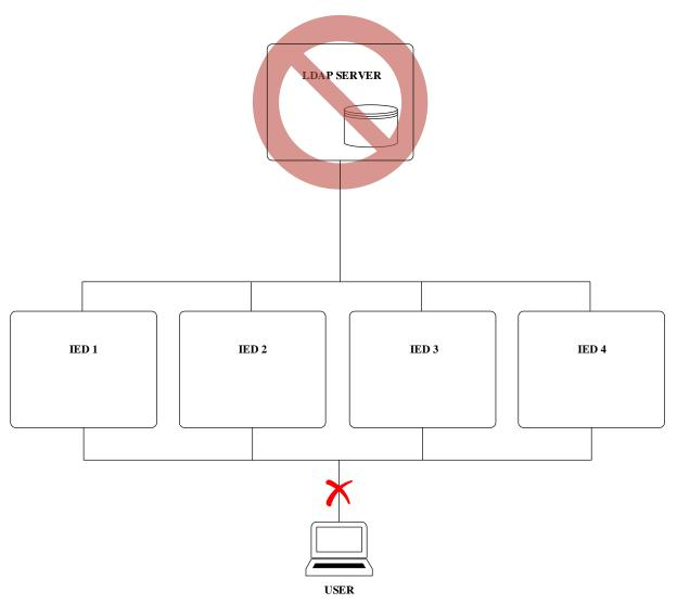
Figure 3.5.1 Logical drawing of a single LDAP server setup
