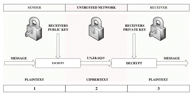
Figure 2.2.2 Asymmetric encryption and decryption process
