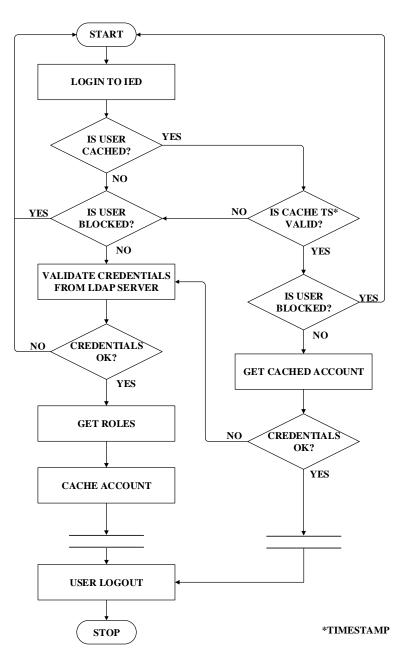
Figure 3.6.2 Logic diagram for caching a user account
