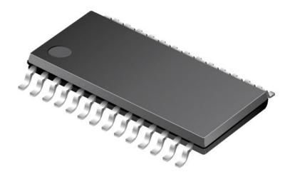
Figure 4.2.1 Trusted Platform Module (TPM) [21]
