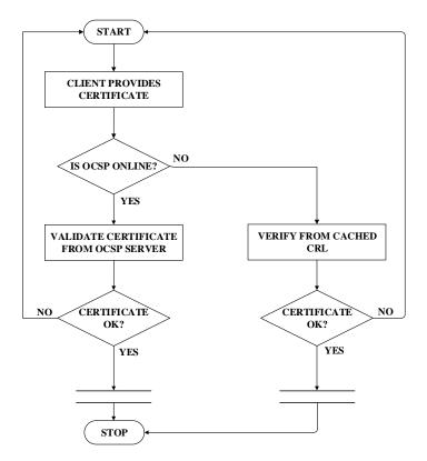
Figure 4.4.2 Logic diagram for certificate verification
