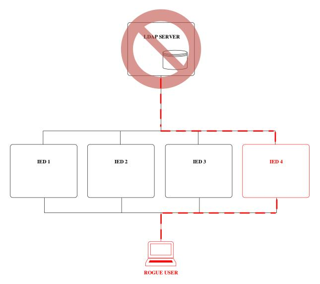
Figure 3.6.1 A rogue user in a substation communication network
