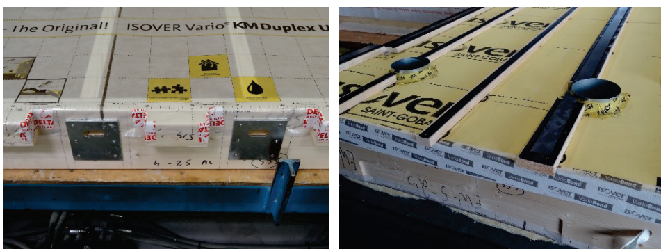
Figure 4.24 All joints and connections were properly sealed at the factory from interior side (left) and from exterior side, including penetrations of ventilation ducts (right) (2017).
