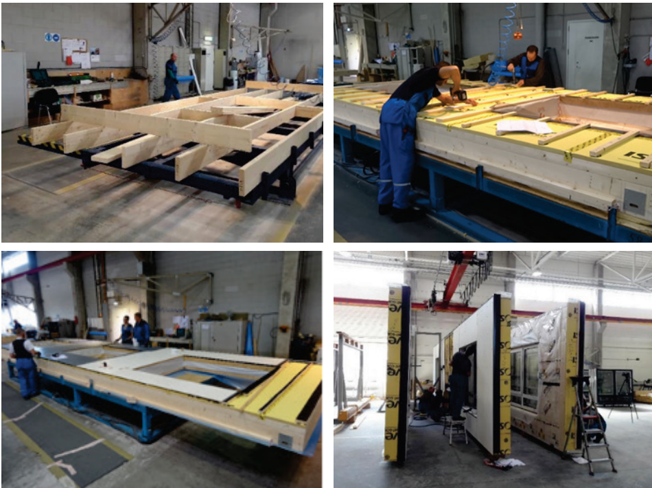
Figure 4.20 Production of elements at the factory of AS Matek in 2017. Preparation of timber framing for insulation (top left), fixing of MW wind barrier boards and ventilated air gap battens (top right), mounting of facade boards (bottom left) and windows (bottom right).
