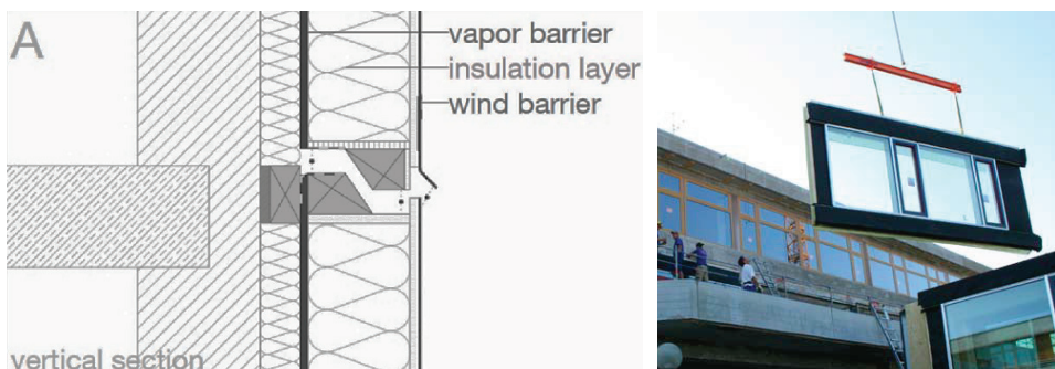
Figure 2.3 Vertical section of the principal design of a TES element (left) (Loebus et al. 2014). Mounting of TES elements in Finland (right) (Lattke et al. 2009).
