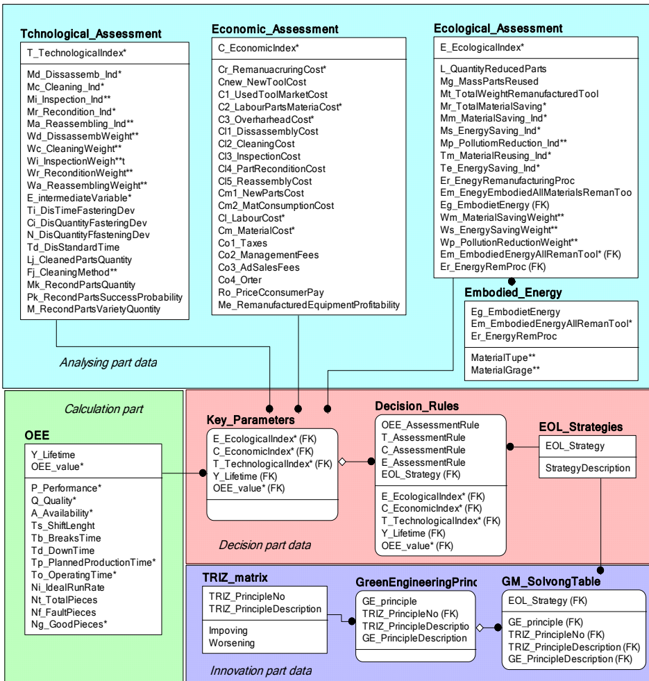
Figure 3.10 Framework of database architecture
