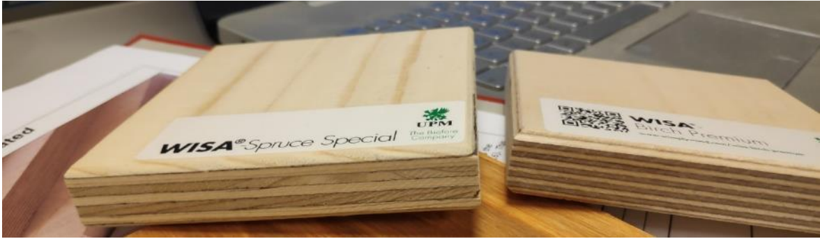
Figure 2 Wisa Company plywood samples, left one from 5 layer of 3 mm spruce veneers and right one is from 11 layers 1.5 mm birch veneers [5]
