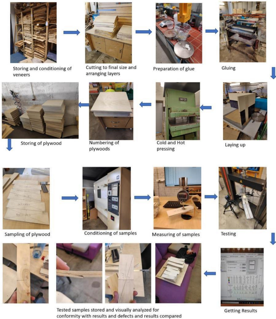
Figure 6 Plywood production and specimen testing steps from log yard to tested specimens
