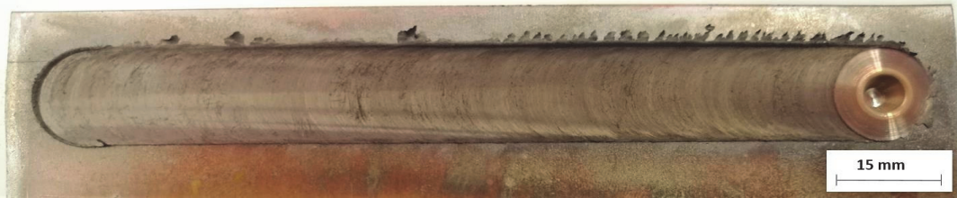
Fig. 2 Image of the visually macroscopic defect-free weld of copper.
