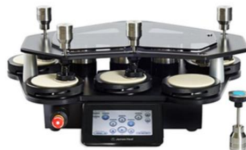
Figure 4.4 James Heal mini Martindale machine for abrasion test [58]
