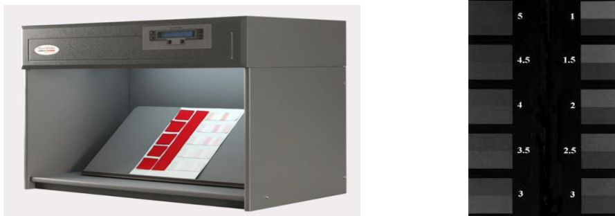
Figure 4.2 Evaluation done by the colour assessment cabinet and evaluation scale [57]
