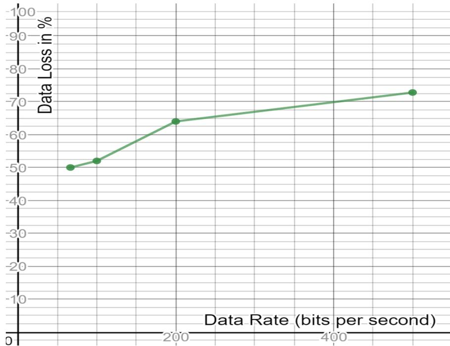
Figure 30 Shows the graph for Data Loss Vs Data Rate for system without Manchester coding
