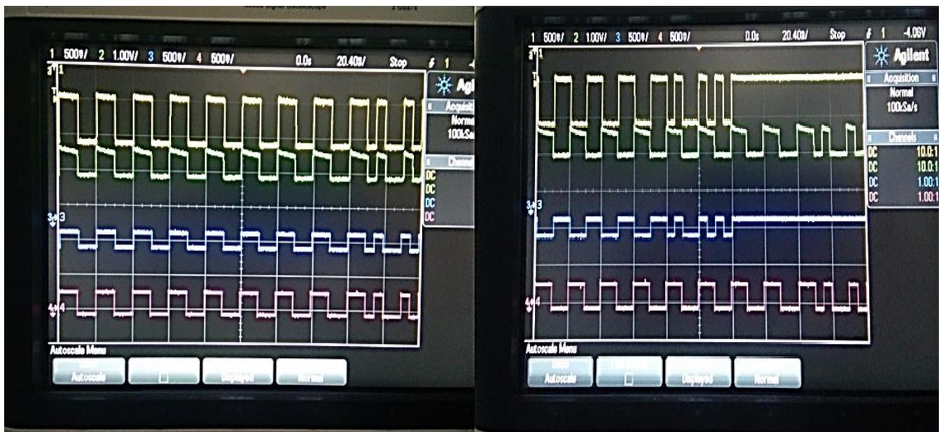
Figure 33 Shows the Output at all TX and RX on the three nodes in prototype 2. The left and right images represent different interval of time.
