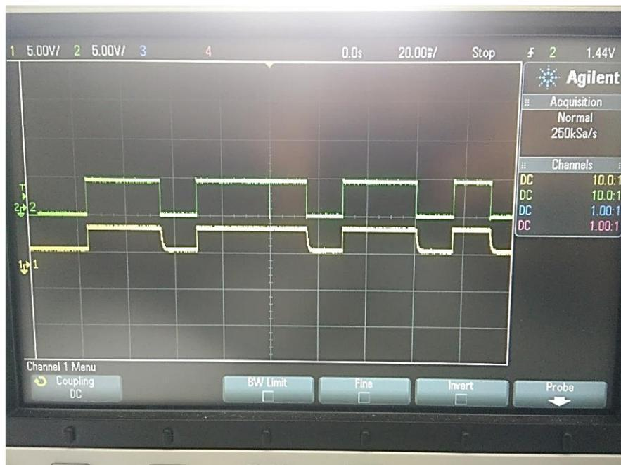
Figure 27 Shows the outputs of Tx and Rx on the oscilloscope for the system without Manchester Coding.
