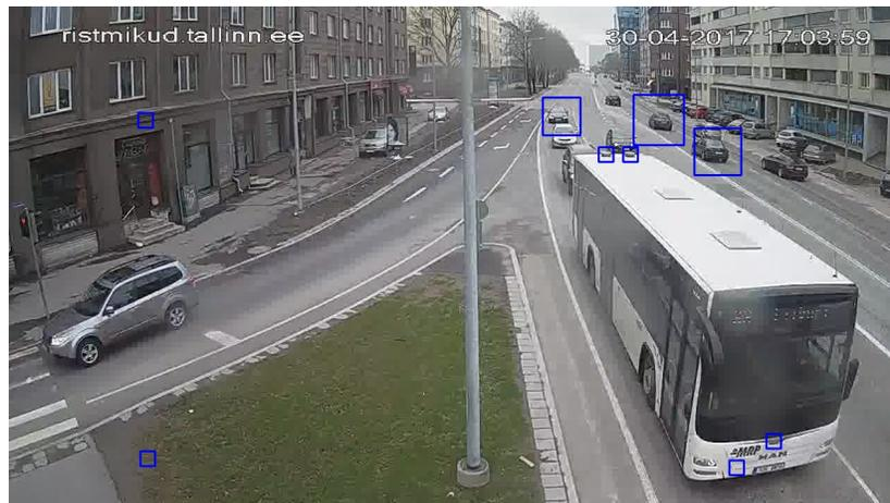
**Figure 11:** Using Haar cascades, false-positives are often more numerous than true-positives. Because many false detections are very small in scale, limiting the minimal detection size might help.
