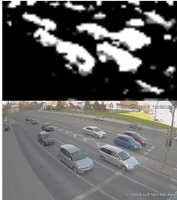
**Figure 16:** The model produces a map of class probabilities from the input image. Top image displays the predictions of class "vehicle" from the bottom image.
