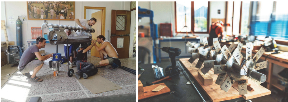
Fig. 3: Snapshots from the manufacturing process of a grinder for aromatic plants, utilising locally sourced scraps.
