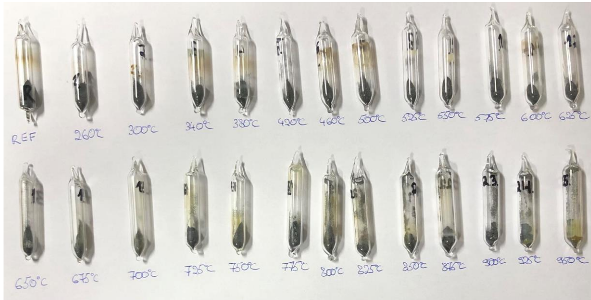
Figure 2.1 \text{Cu}_2\text{ZnSnS}_4 powders sealed in quartz ampoules post anneal.
