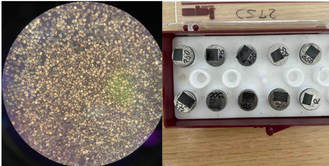
Figure 2.5 An optical microscope picture of the measured monograins on the left and the samples S700-S950 with the reference sample in a holder.
