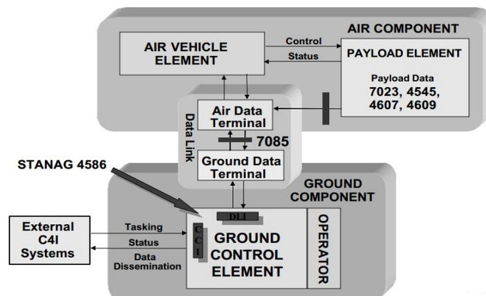
Figure 3: STANAG for UAV control [8]
