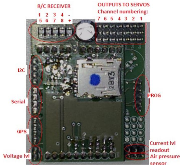
Figure 13: AKPilot connections
