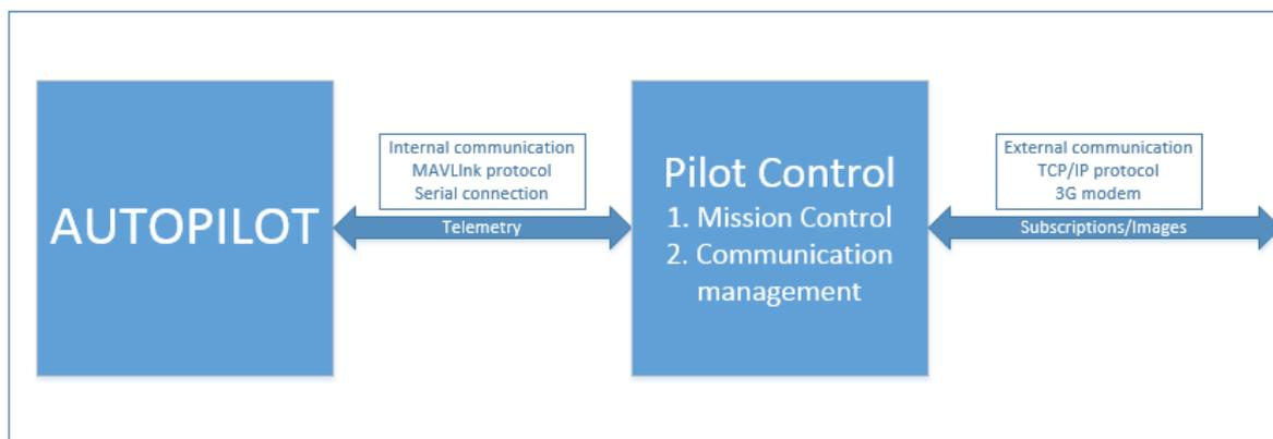
*Figure 20: Internal and external communication model*
