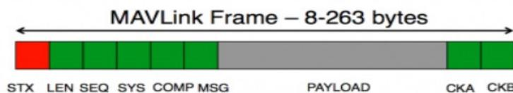
*Figure 4: MAVLink packet structure [12]*
