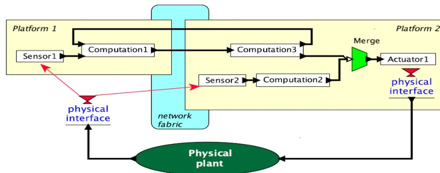
*Figure 8: Structure of a cyber-physical system [22]*
