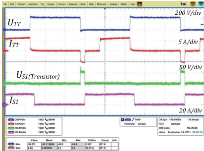
Fig. 8. IGBT voltage and current (top), S1 MOSFET voltage and current (bottom) of the experimental converter prototype.
