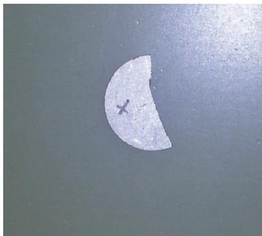
**Figure 48. Damaged PZT transducer**
