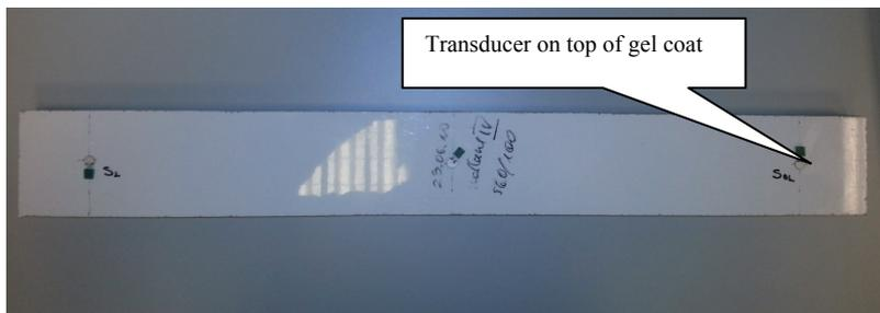
**Figure 44. Photo of a test specimen with PZT transducers**
