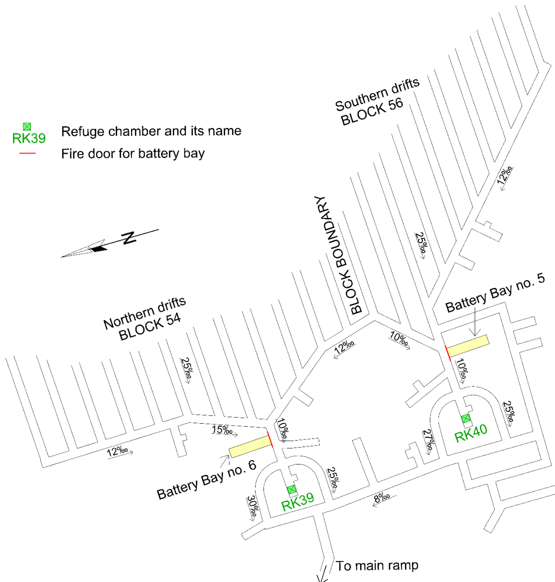
Figure 4.10 Location of the refuge chambers on level 536
