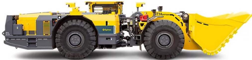
Figure 3.4 Epiroc's ST14 Battery loader (Epiroc, n.d.b)
