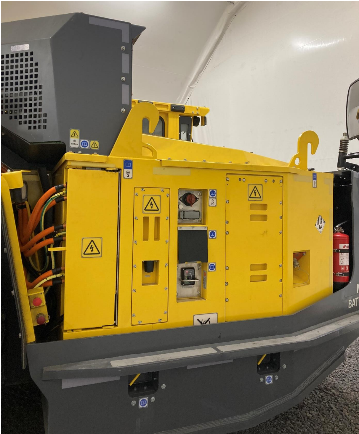
Figure 4.1 Main battery of the MT42 Battery truck
