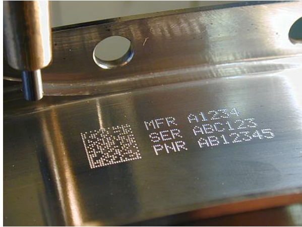
Figure 2.9. Dot peen marked detail [29]
