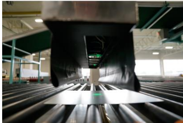
Figure 2.2. Datalogic Matrix 300N 2D imager for industrial applications [9]
