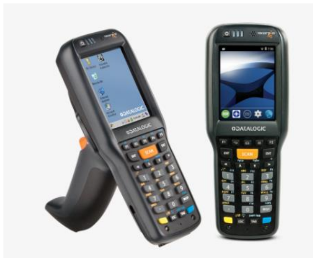
Figure 2.3. Datalogic Skorpio X4 hand-held 1D barcode scanner [10]
