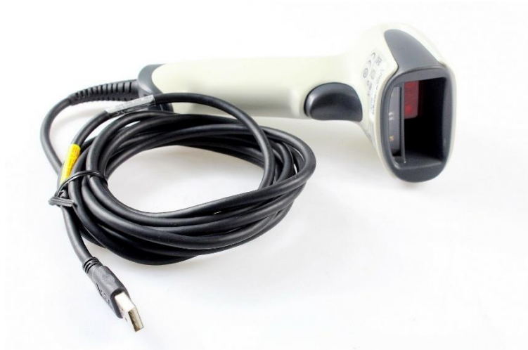
Figure 3.2. BS-970 hand-held laser scanner [40]
