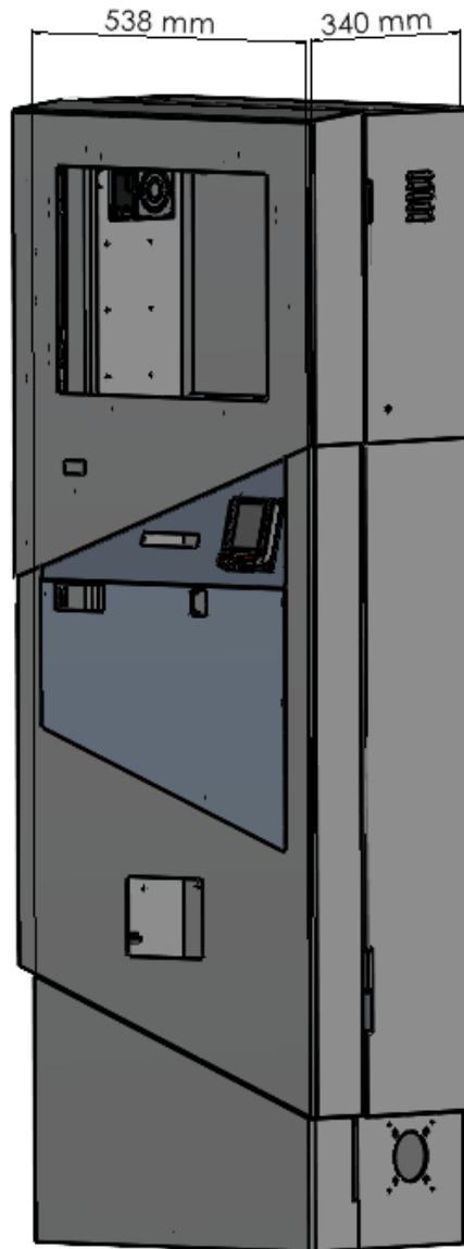
Figure 1.1 Overview of the generation 1 payment kiosk 3D model along with its internal dimensions
