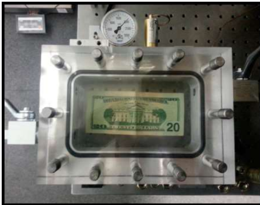
Figure 5. High pressure CO 2 cell in the supercritical phase (60 °C, 2000 psi) [27].
