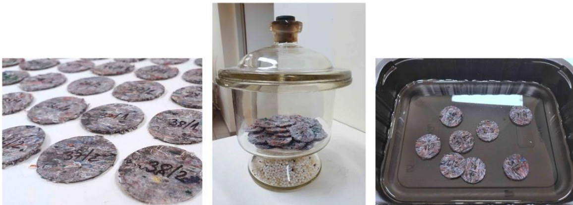
Figure 28. Measuring and conditioning the test specimen for water uptake test
