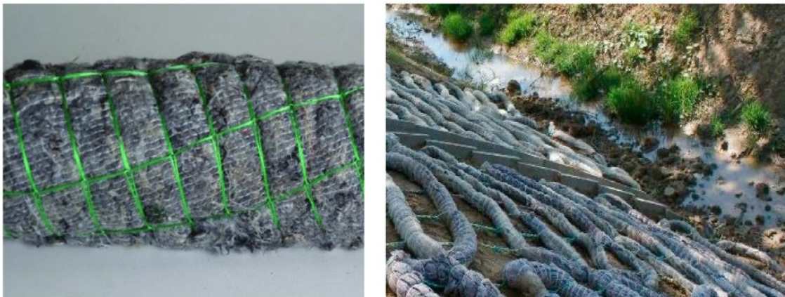
Figure 13. The Kemafil rope manufactured from the nonwoven made from blended recycled fibres (left) [61] and the ropes arranged meandrally on the surface of the steep slope in a gravel pit [62]
