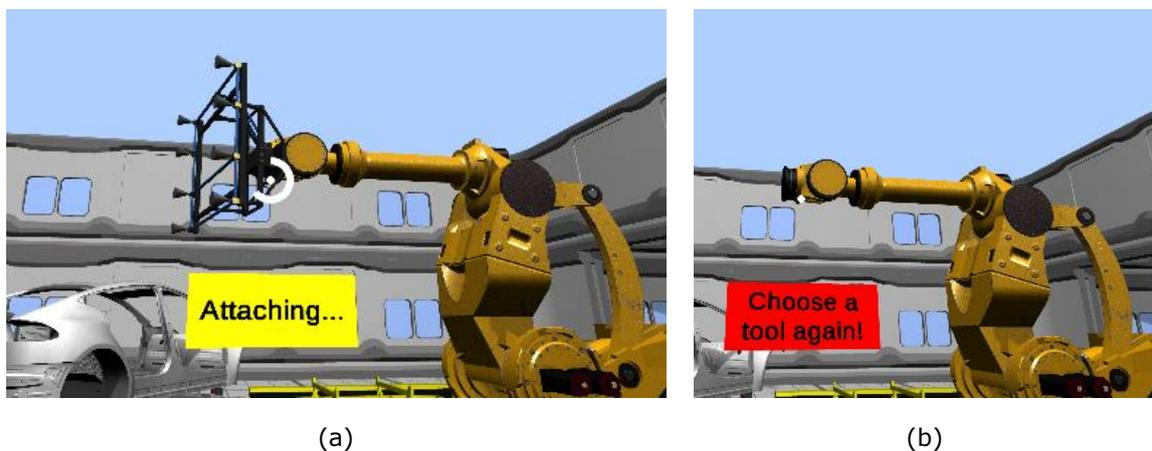
Figure 4.10. Tool being attached to the industrial robot (a) and message informing the user that a new tool must be selected (b)
