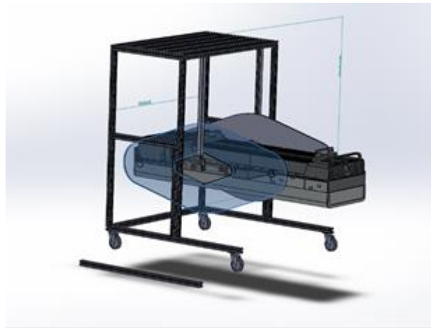
Figure 7 Design 1 (Trolley Lift)
