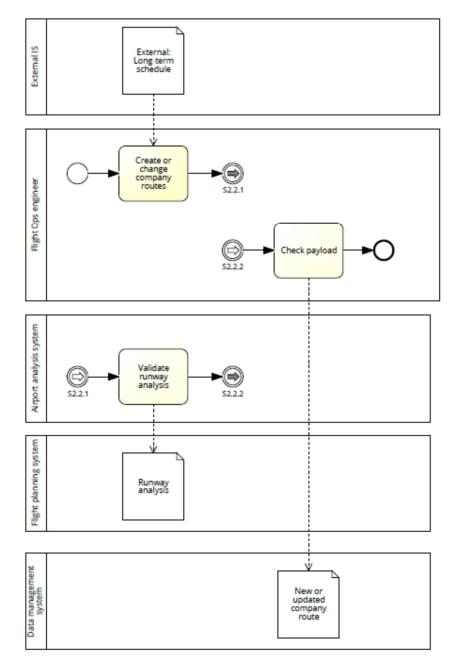
Figure 18. Company routes management subprocess, expanded. (Rein Nõukas)
