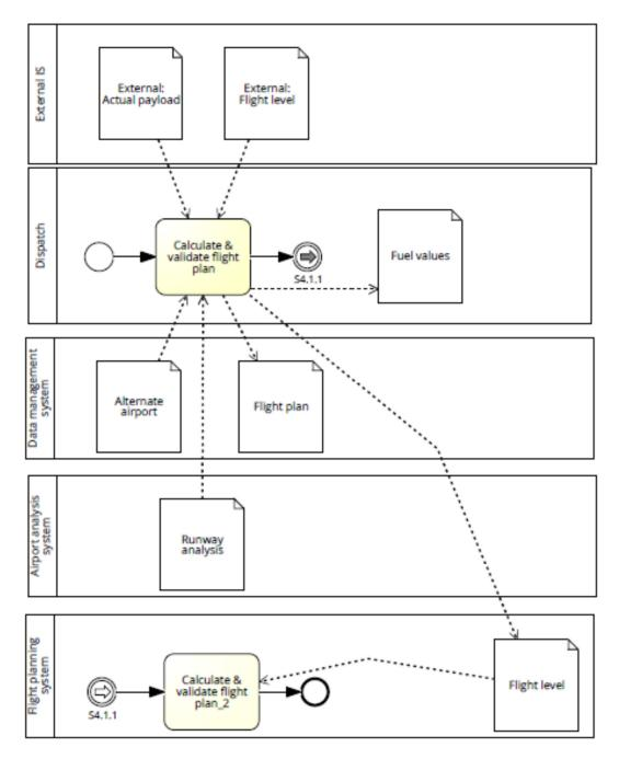
Figure 37. Flight plan calculation & validation subprocess, expanded. (Rein Nõukas)
