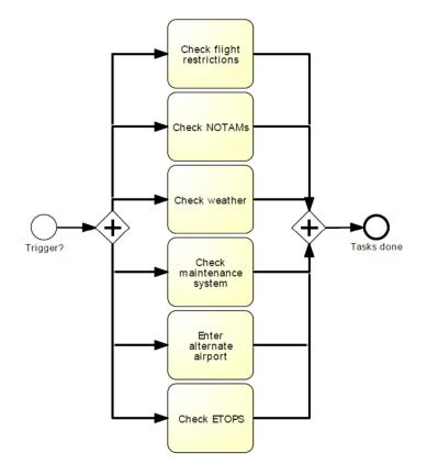
Figure 33. Dispatcher tasks, expanded – a sublayer of Dispatcher operations subprocess. (Rein Nõukas)
