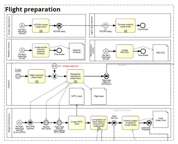
Figure 46. Flight preparation as one of the phases of the day of operation. (Rein Nõukas)
