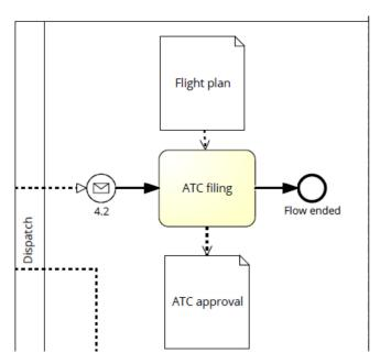
Figure 40. ATC filing workflow. (Rein Nõukas)
