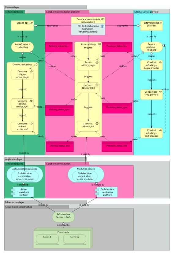
Figure 54. The coordination part of the collaboration mechanism. (Rein Nõukas)
