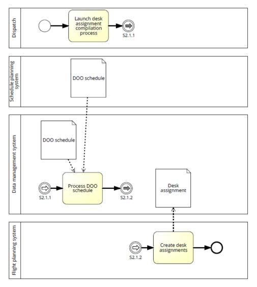
Figure 24. Desk assignment compilation subprocess, expanded. (Rein Nõukas)
