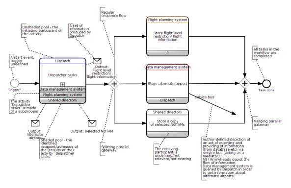
Figure 6. Dispatcher operation subprocess. (Rein Nõukas)
