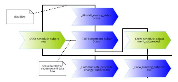
Figure 44. Depicting data and sequence flows in a value-chain model. (Rein Nõukas)
