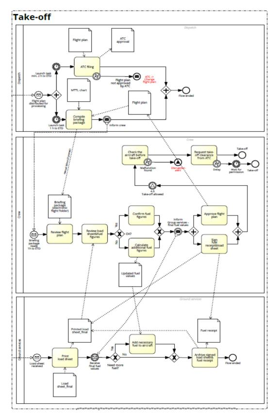
Figure 48. Take-off as one of the phases of the day of operation. (Rein Nõukas)
