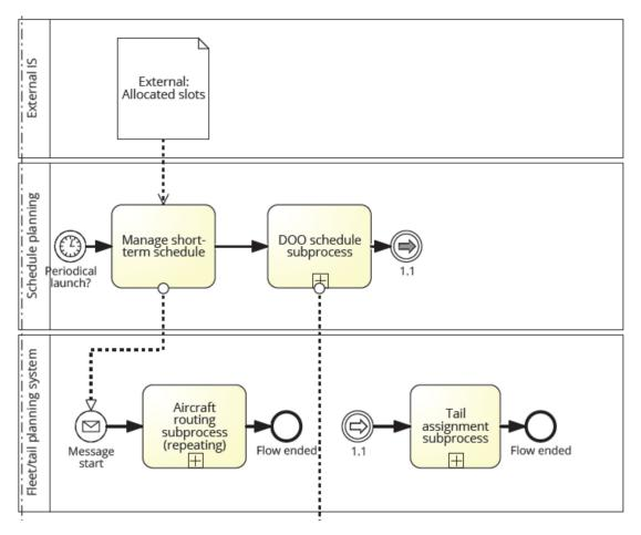
Figure 14. Scheduling and tail assignment workflow. (Rein Nõukas)
