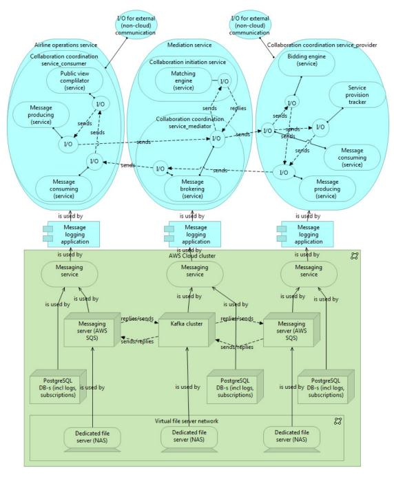
Figure 57. The abstract architecture of the collaboration mechanism. (Rein Nõukas)
