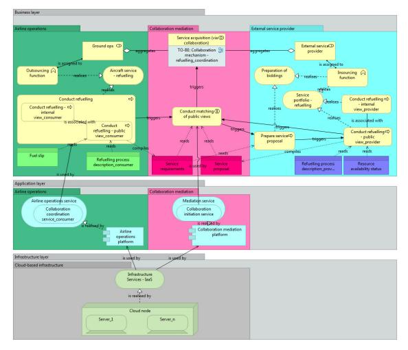
Figure 53. The bidding part of the collaboration mechanism. (Rein Nõukas)
