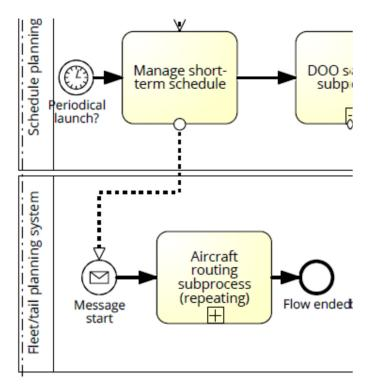
Figure 10. Aircraft routing workflow. (Rein Nõukas)
