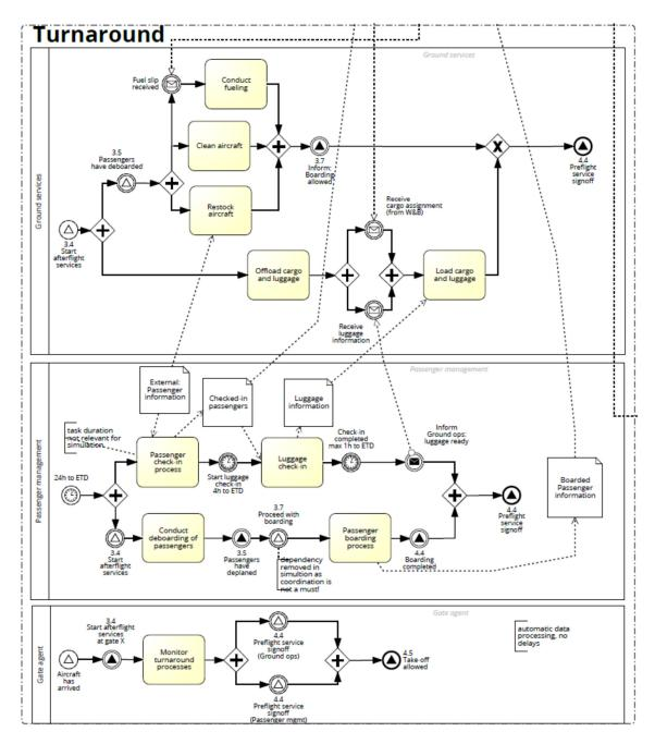
Figure 47. Turnaround as one of the phases of the day of operation. (Rein Nõukas)
