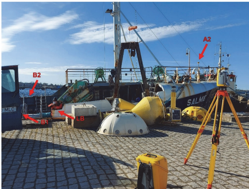
Figure 3: Total station survey for coordinating the ARPs (A2) and benchmarks on the vessel's railing (B1, B2, and LB; note that B1 is behind the car).
