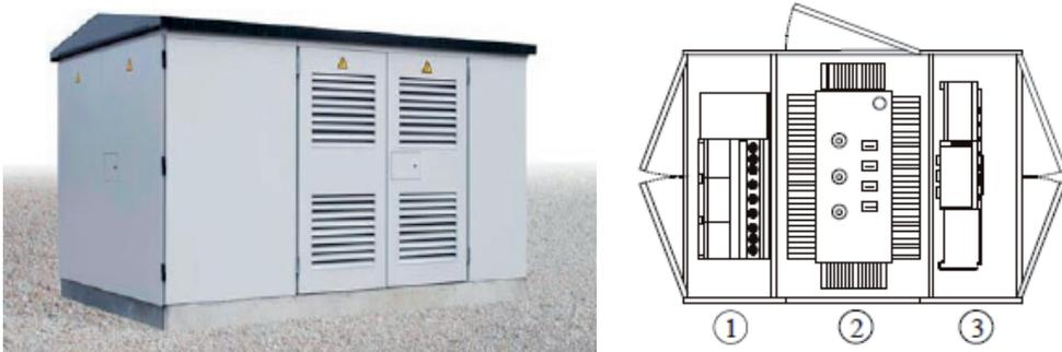
*Fig. 1.30 Example layout of 1000 kVA non walk-in prefabricated metal enclosure substation (with MV section – 1; transformer section – 2; LV section – 3) [73]*
