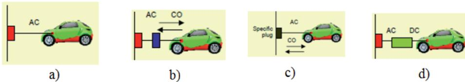
Fig. 1.8 Charging modes according to IEC 61851 [56]
