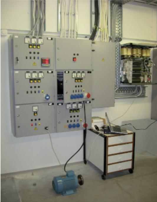
*Fig. 5.14 Test set-up with electric motor in the no-load state with bidirectional AC-DC converter operating in parallel*
