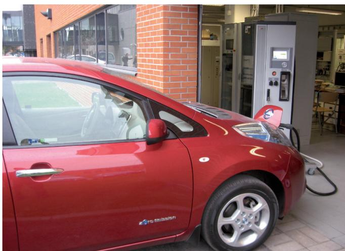
Fig. 5.17 Test set-up with EVSE with bidirectional AC-DC converter operating in parallel
