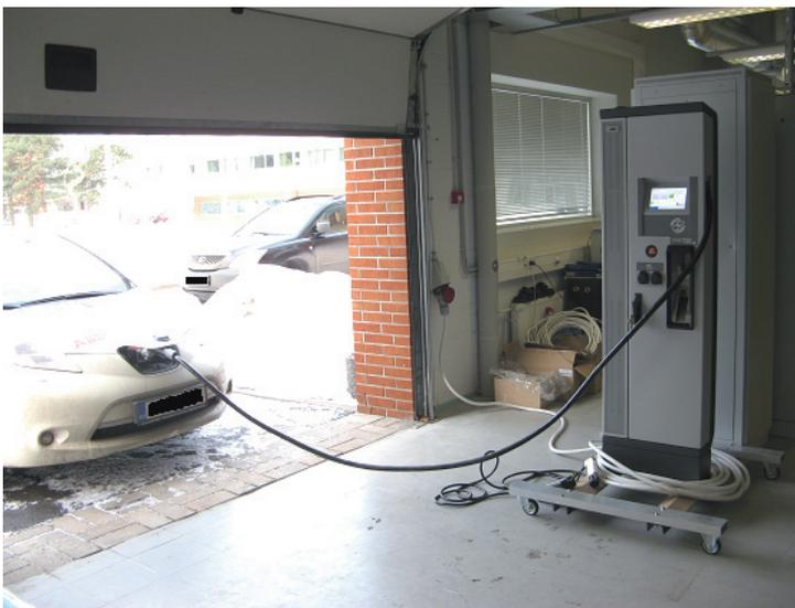
*Fig. 5.5 Fast charger TERRA SC Duo (charging of serial electric vehicle in TUT Department of Electrical Engineering)*
