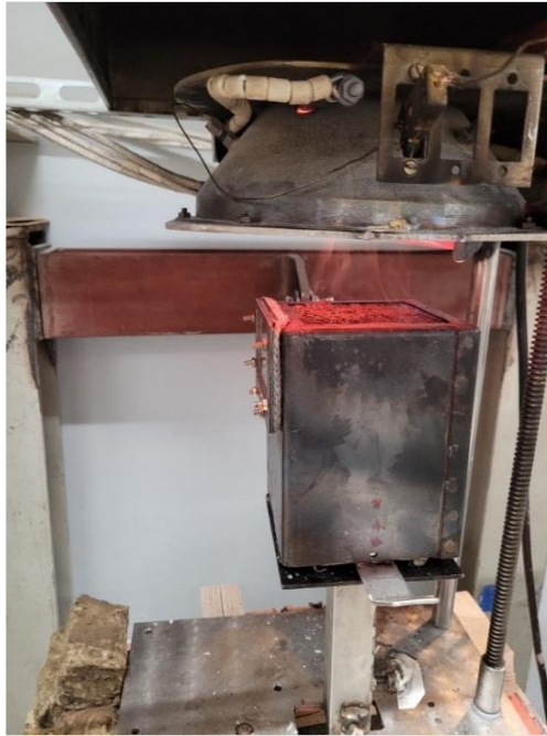
Figure 3.4 Reaction to fire test using cone heater
