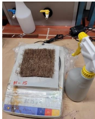
Figure 3.2 Fire retardant treatment spraying technique
