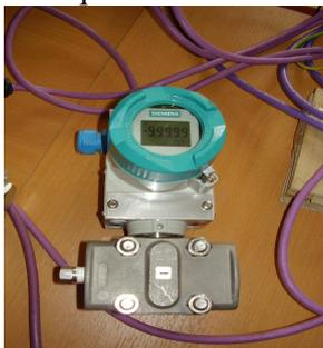
Fig. 3.16 Level transmitter
