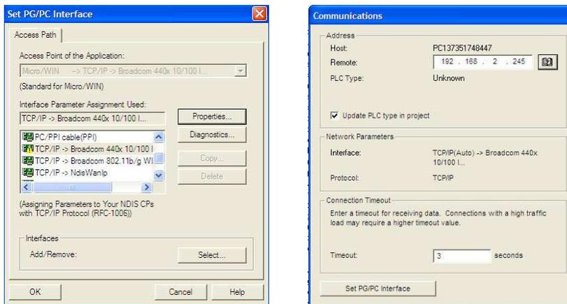
Fig. 19 Windows of the controller address.
