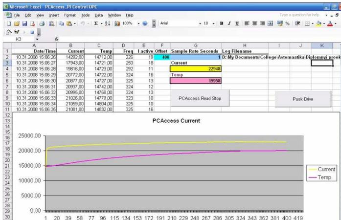
Fig. 23 Graphical display of PLC variables via Excel as OPC client with PC Access as OPC server.
