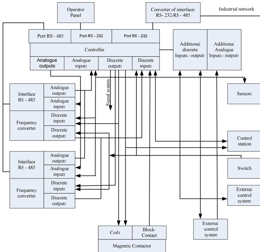
Fig. 1.6 PLC I/O channel specifications.
