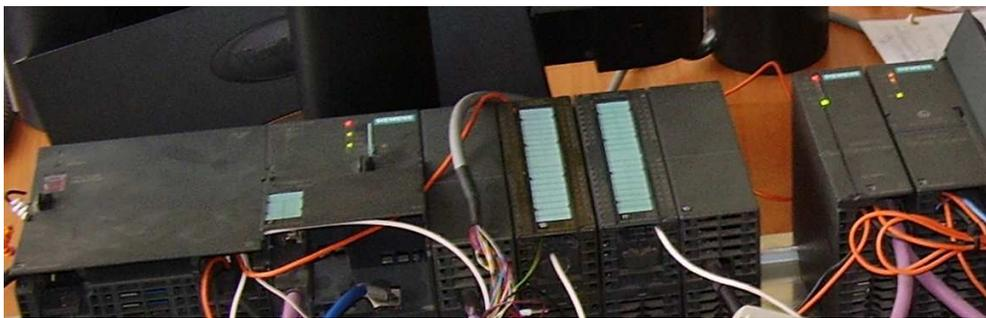
*Fig. 3.9 PROFIBUS test-bench for five sensors of one tank.*
