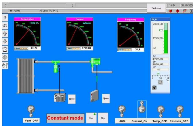
Fig. 22 Current control monitoring.
