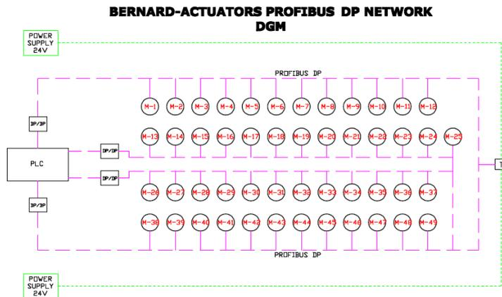
Fig. 3.5 Configuration PROFIBUS for Bernard actuators.
