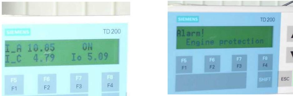
Fig. 14 Current parameters and alarm signals of the Text Display TD200.
