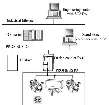
Fig. 2.2 Integration of DP/PA coupler in a system.
