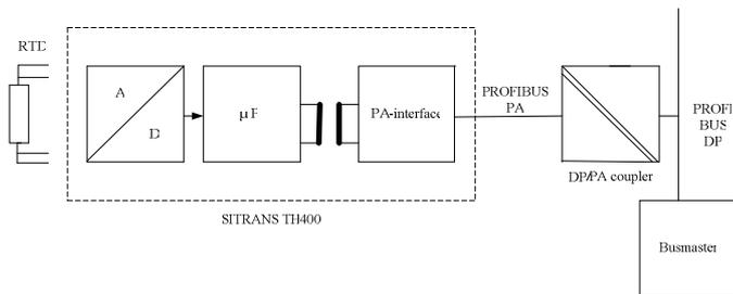
Fig. 3.18 Intelligent sensor SITRANS TH400.
