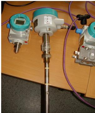
*Fig. 3.14 Pointek CLS 300 level switch.*
