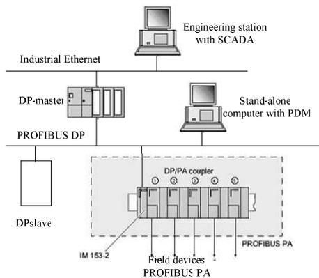
Fig. 2.1 Configuration of the control system network PROFIBUS.
