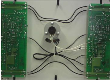
*Fig. 10 Inclinometer for the heel angle measurement.*
