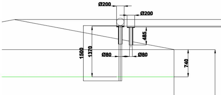
Fig. 3.15 The level switch installation.
