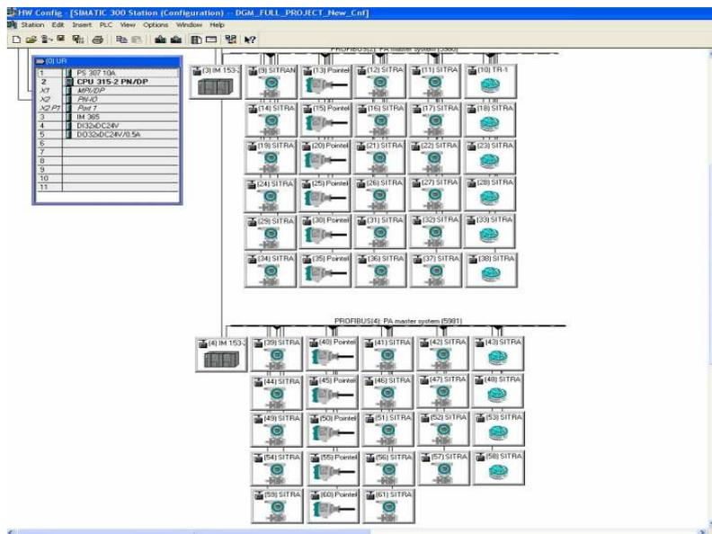
Fig. 3.3 PROFIBUS network configuration for sensors in 10 storage tanks.
