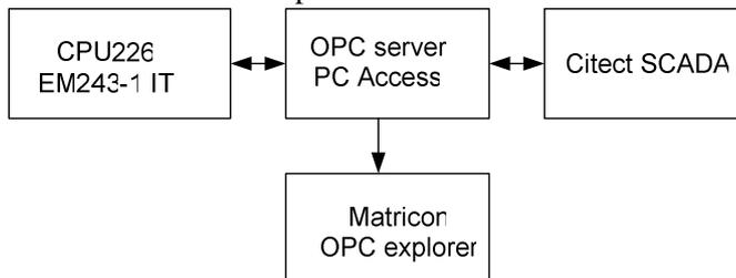
*Fig.1 Block diagram of the controller connection.*
