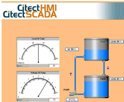
Fig. 6 Liquid level monitoring.
