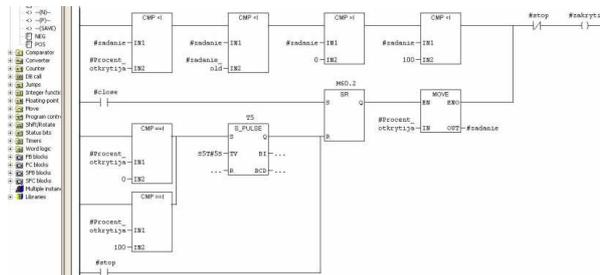
Fig.4.15 Part of the program for valve closing.
