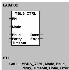
*Fig. 21 Exchange initialization block.*
