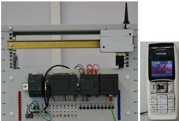
Fig. 16 Set-up with a GSM modem.
