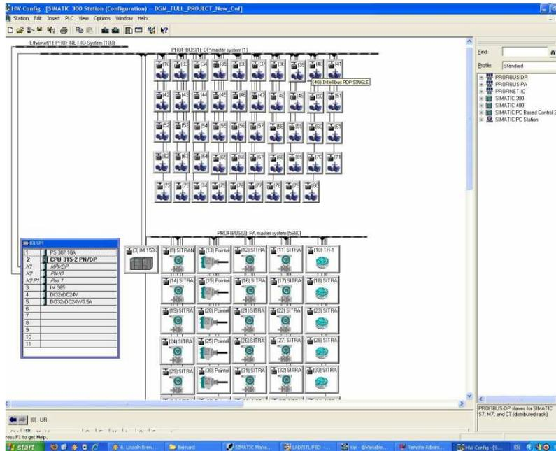
Fig. 3.4 PROFIBUS network configuration for 49 actuators.
