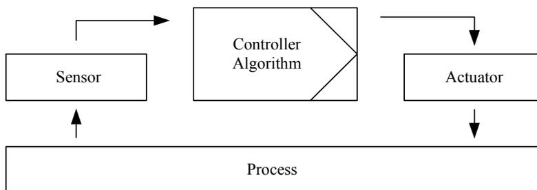
Fig. 1.2 Basic flow of signals in a controller.
