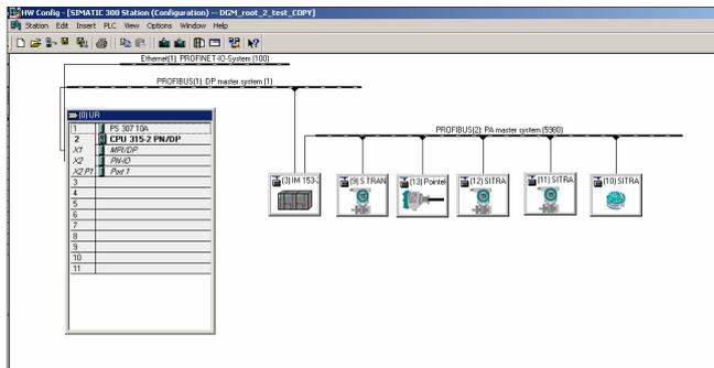
Fig. 3.11 DP-master system in the hardware configuration.
