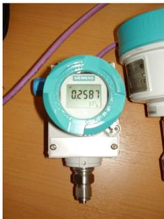
Fig. 3.12 SITRANS P DS III transmitter.
