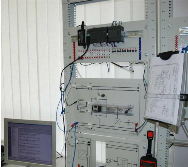
*Fig.2 Set-up for the temperature process control*
