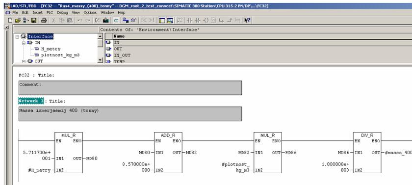
Fig. 4.10 Reference to a local variable by means of symbol addressing.
