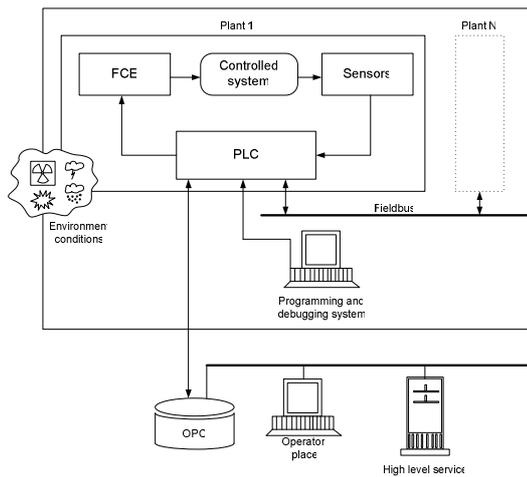
Fig. 1.5 PLC place in the industrial environment.
