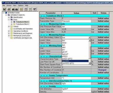
Fig. 3.17 Parametrization in PDM.
