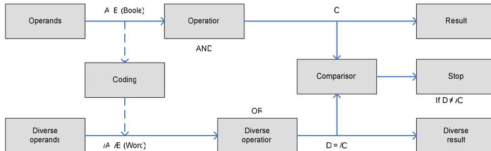
Fig. 1.10 Principle of diverse instruction processing with inverse logic.
