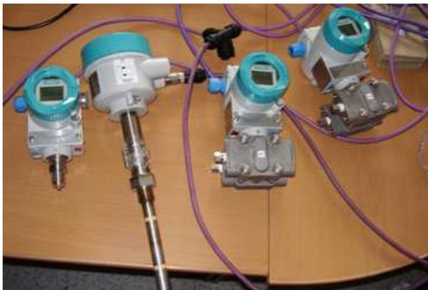
*Fig. 3.10 PROFIBUS PA field devices.*
