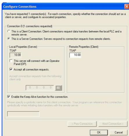
Fig. 18 Address window for the external device TSAP.
