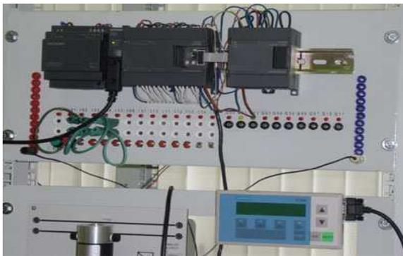
*Fig. 13 PLC with the Text Display TD200.*
