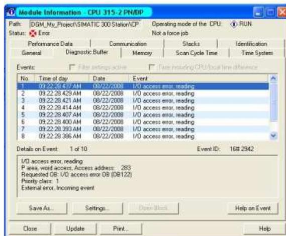
Fig. 4.17 Interpreting error messages in the diagnostic buffer.
