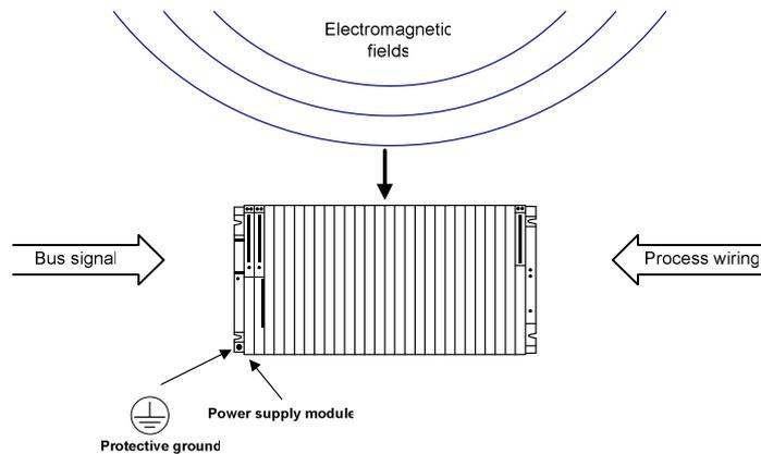
*Fig. 1.11 Possible routes for electromagnetic interference.*
