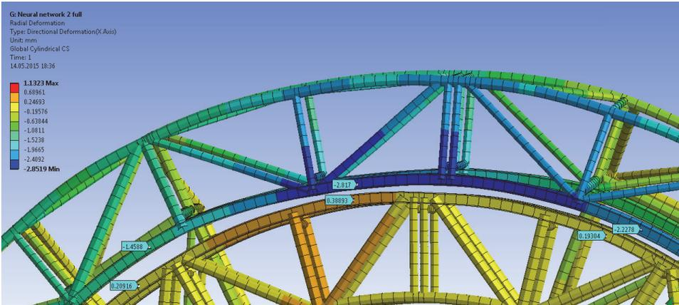
Figure 3.7. The rotor's and stator's air-gap deformations.
