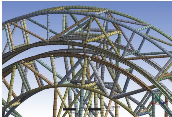
Figure 3.5. Structural mesh with beam elements.
