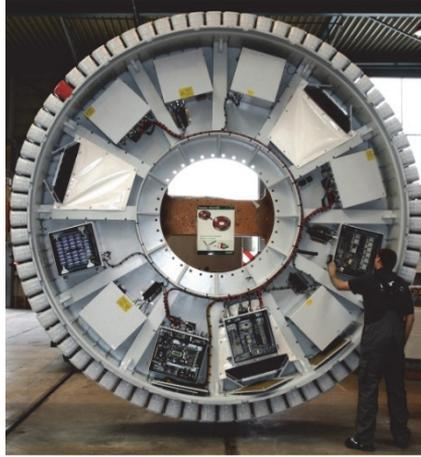
*Figure 1.8. Radially stiffened rotor structure of Enercon GmbH [53].*
