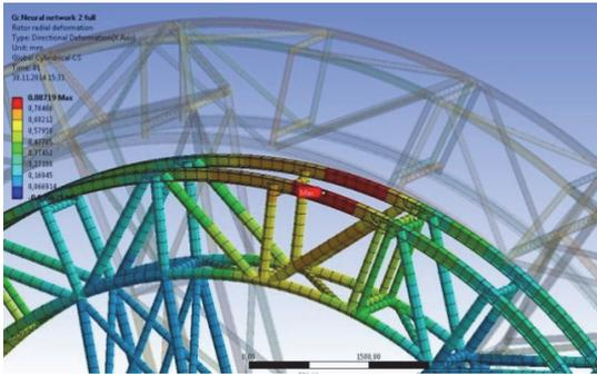
Fig. 4. FEM model of the generator.
