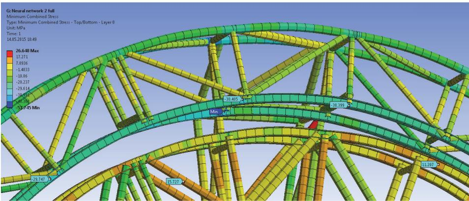
Figure 3.8. The rotor's and stator's minimum combined stress.
