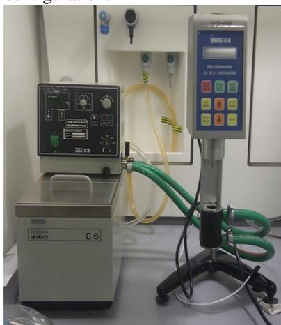
[C] Concentric cylinder viscometer Brookfield RVDVII+.
