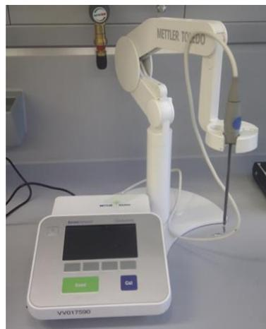
[D] Electrical conductivity meter SevenCompact Conductivity S230.
