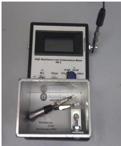
[F] Membrane electrical conductivity meter.
