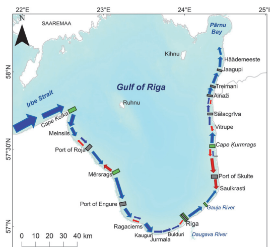
Figure 13. Transport directions (arrow widths correspond to the rate of potential net transport), major interconnected sedimentary compartments separated by major natural divergence points of net sediment transport (green rectangles), and large harbours and jetties (black rectangles) that split the sedimentary compartments into almost separated cells. Blue arrows indicate counter-clockwise transport, and red arrows show clockwise transport. Parallel narrow blue and red arrows denote the variable transport regime in different years.
