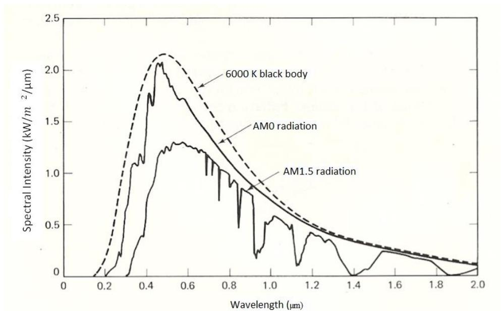
Figure 2.9: Spectral distribution-wavelength graph depending on the air mass [10].
