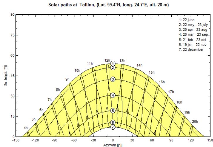
Figure 4.6: Sun path diagram at Tallinn
