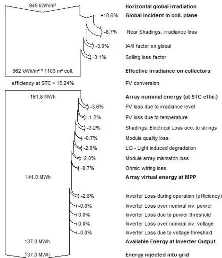
Figure 4.17: Shading Loss diagram in PVsyst
