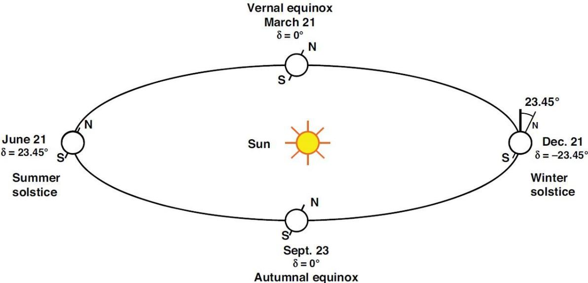
Figure 2.3: The Earth's orbit around the Sun and the position of the Earth's axis over the course of a year [5].
