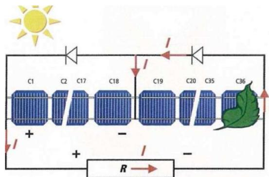
Figure 4.14: Bypass diode on solar cell [17]
