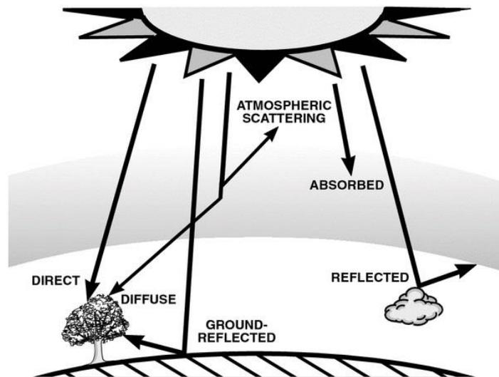
Figure 2.7: The total global radiation on the ground has direct, scattered and reflective components. [8]
