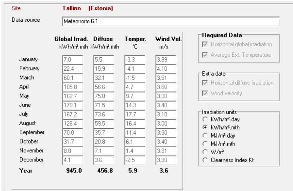
Figure 4.7: Monthly meteorological data used in PVsyst.
