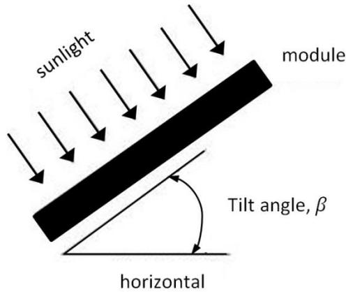
Figure 4.10: Illustration of module tilt angle.
