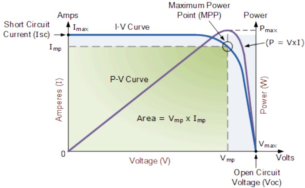
Figure 3.4: I-V and power curves of a solar cell [14].
