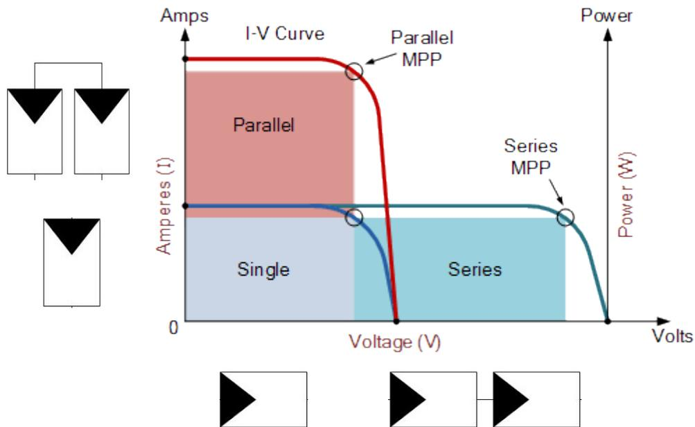
Figure 3.5: Interconnection of PV modules [14].
