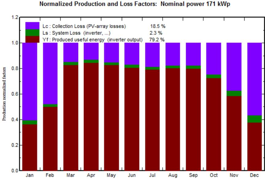
Figure 6.3: Scenario M1-4 monthly normalized production and loss factors
