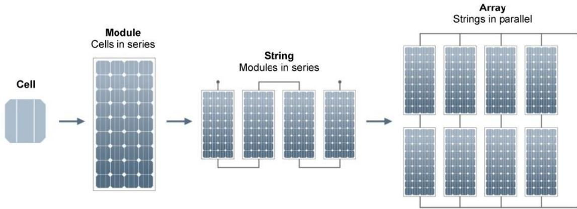
Figure 3.2: Solar cell, PV module, string and array [13].
