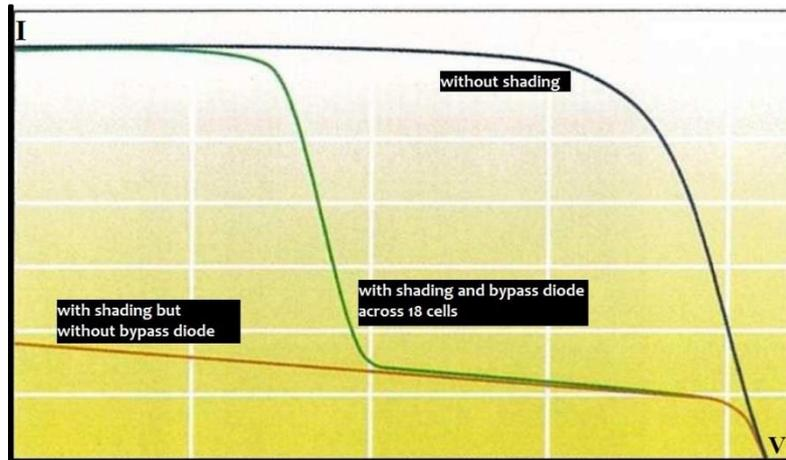
Figure 4.15: Module characteristic I-V curves with and without bypass diodes [17]
