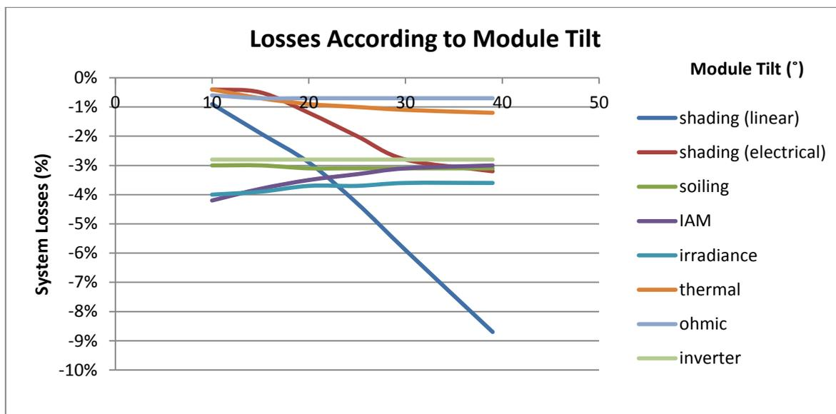
Figure 6.1: Simulation-P1 Losses according to module tilt
