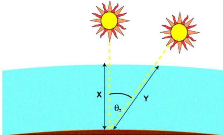
Figure 2.8: The air mass represents the proportion of atmosphere that the light must pass through before striking the Earth relative to its overhead path length, and is equal to  $Y/X$  [9].
