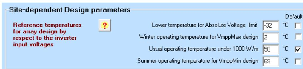
Figure 4.9: Site-dependent design parameters in PVsyst.
