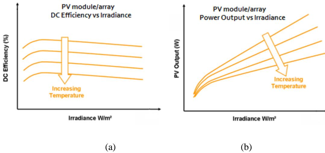
Figure 3.7: PV module/array DC Efficiency-Irradiance (a), Power Output-Irradiance (b) [15].
