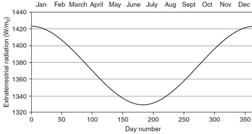
Figure 2.6: Variation of extraterrestrial solar radiation with the time of year [6].
