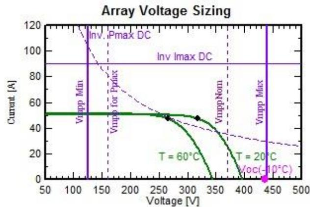
Figure 4.16: PV array I-V curves and an inverter's operating range
