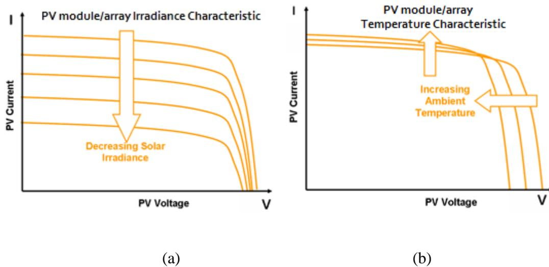
Figure 3.6: PV module/array Irradiance (a), Temperature (b) Characteristics [15].
