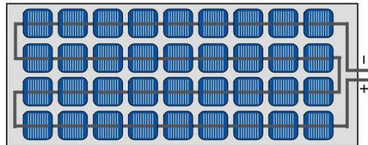
Figure 3.3: Solar cells in series connection [9].
