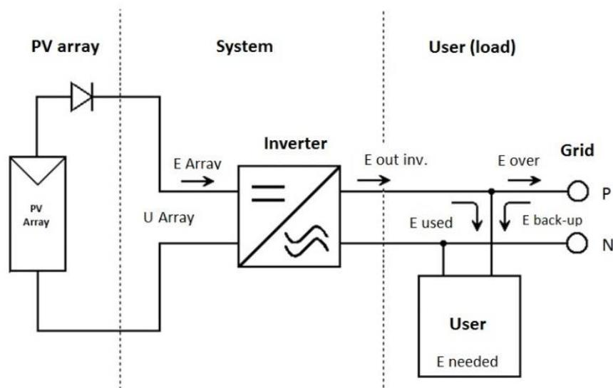
Figure 3.1: Simplified schema of a grid-connected PV system
