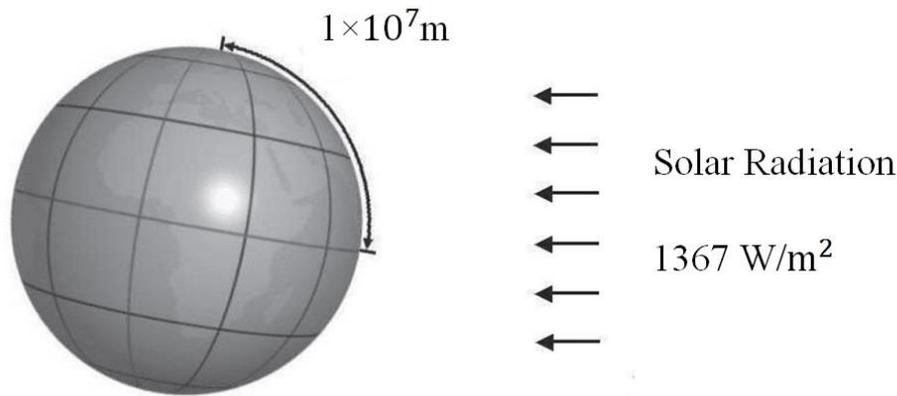
Figure 2.1: Solar constant and length of the meridian from the North Pole to the equator [3].
