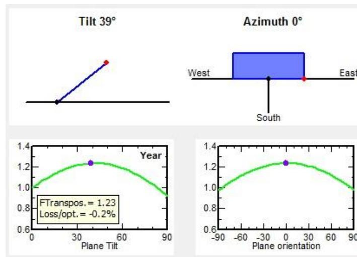
Figure 4.11: Transposition factor as a function of azimuth and plane tilt
