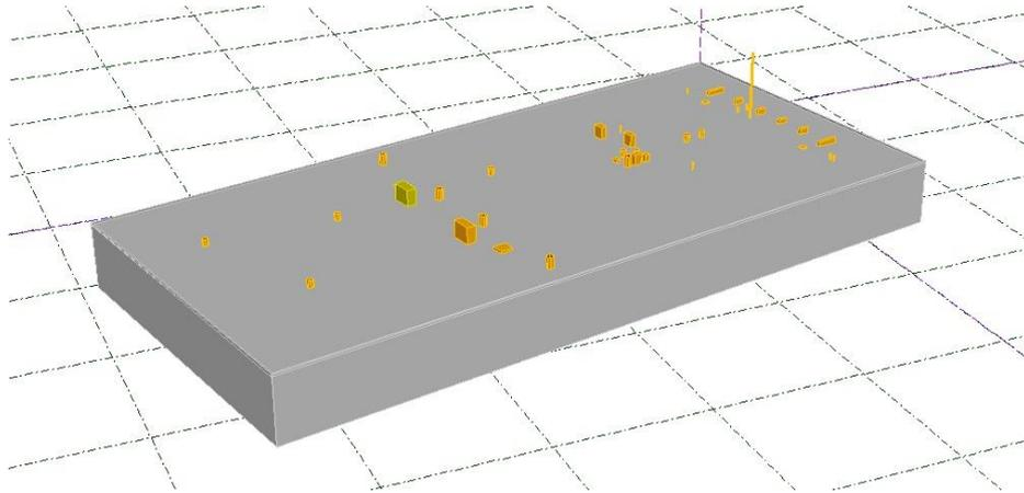
Figure 4.5: 3D representation of the building with shading objects
