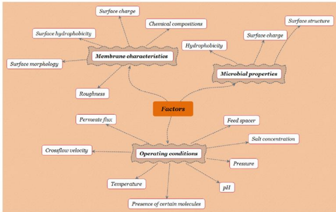
Figure 7: Factors affecting bacteria attachment to membrane surface [2]
